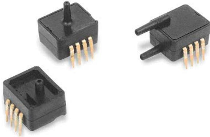
The ASDX series is an amplified version of Honeywell's proven performer and industry leading SDX series sensor. The amplified ASDX sensor's footprint is slightly larger than the SDX but it offers a high level output (4.0 Vdc span) on a very cost-effective basis. This series is fully calibrated and temperature compensated with on-board Application Specific Integrated Circuitry (ASIC). They are intended for use with non-corrosive, non-ionic working fluids; such as air and dry gases.
