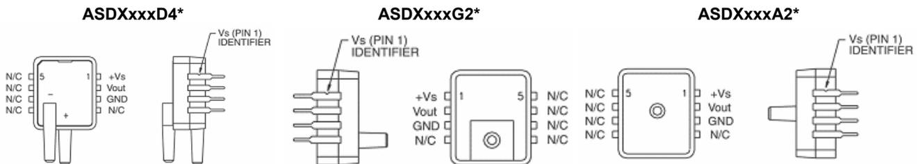
\* N/C means no connection, connecting to ground will damage to sensor.
