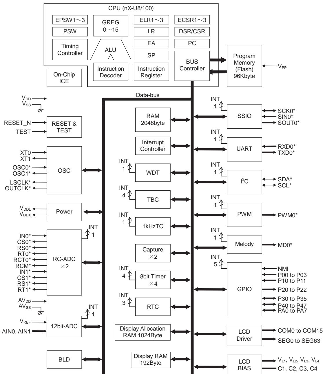
**Figure 1 ML610Q435 Block Diagram**
