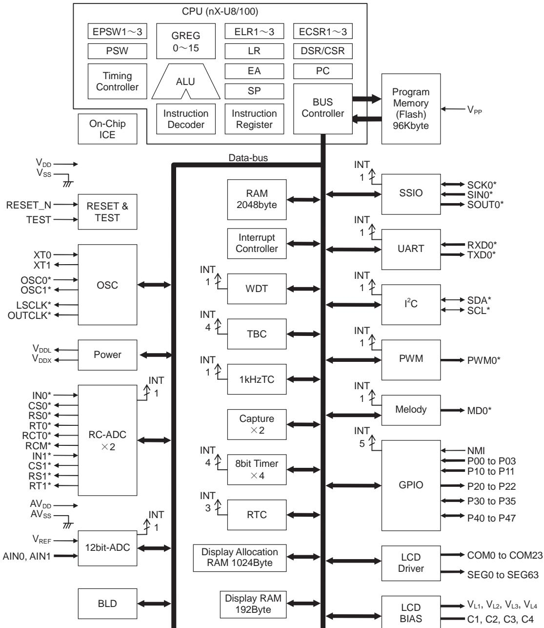
**Figure 2 ML610Q436 Block Diagram**
