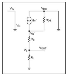
Figure 2. Small-signal model of the Figure 1 circuit.
