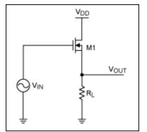
Figure 1. Test circuit for gain measurements.
