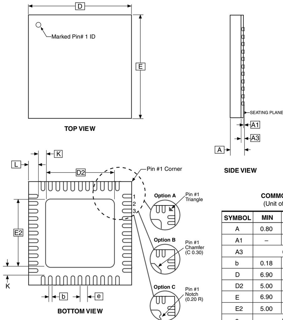
Note: JEDEC Standard MO-220, Fig. 1 (SAW Singulation) VKKD-3.
