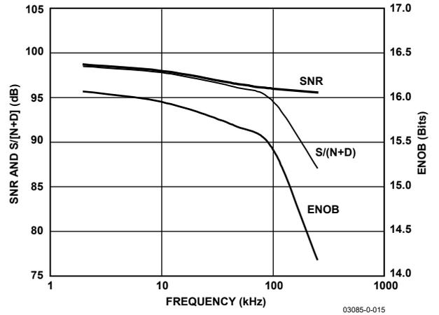
Figure 15. SNR, S/(N+D), and ENOB vs. Frequency
