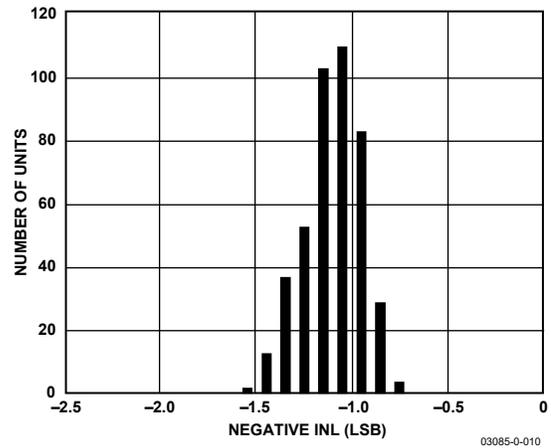
Figure 11. Typical Negative INL Distribution (424 Units)
