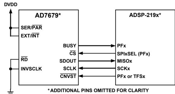
Figure 44. Interfacing the AD7679 to an SPI Interface
