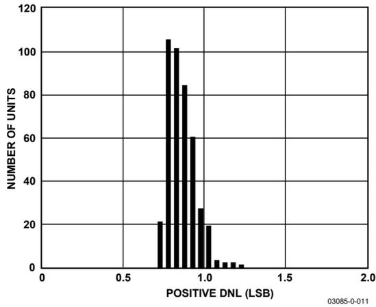
Figure 12. Typical Positive DNL Distribution (424 Units)
