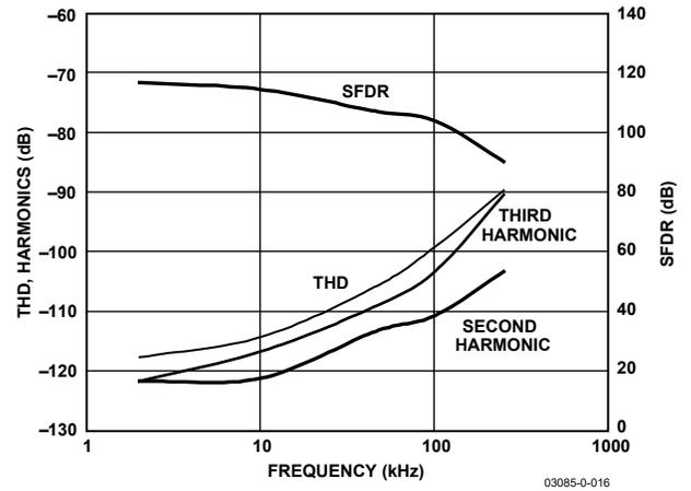
Figure 16. THD, SFDR, and Harmonics vs. Frequency
