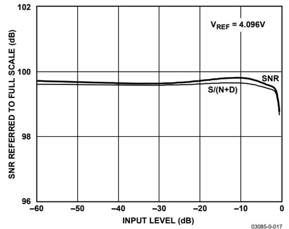
Figure 17. SNR and S/(N+D) vs. Input Level
