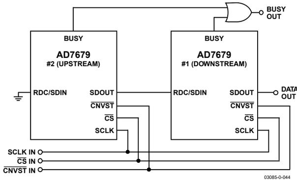
Figure 43. Two AD7679s in a Daisy-Chain Configuration
