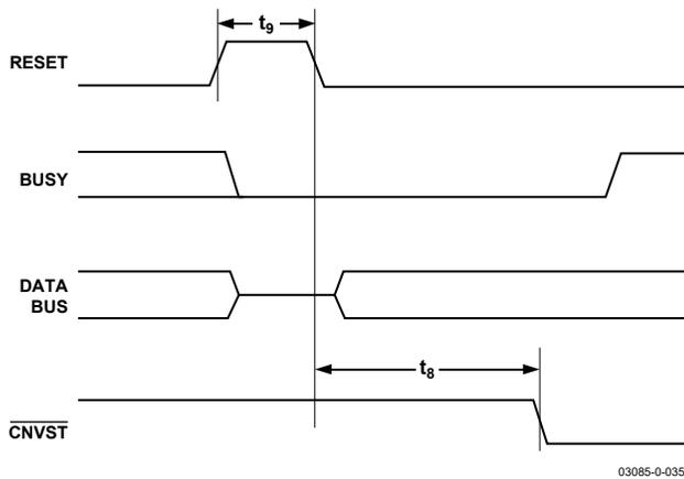
Figure 34. RESET Timing
