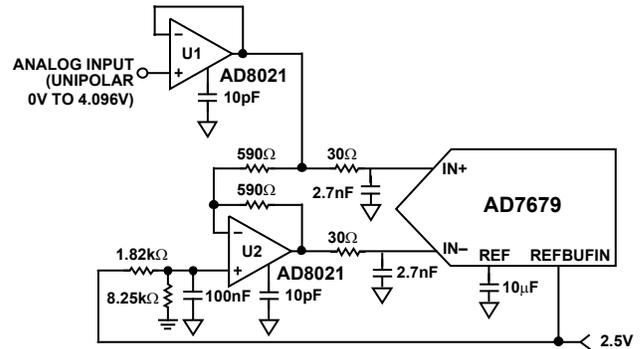
Figure 30. Single-Ended-to-Differential Driver Circuit (Internal Reference Buffer Used)
