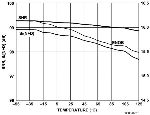
Figure 18. SNR, S/(N+D), and ENOB vs. Temperature
