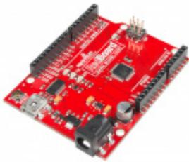
SparkFun RedBoard - Programmed with Arduino
