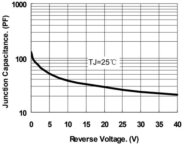
Fig.1-Typical Junction Capacitance
