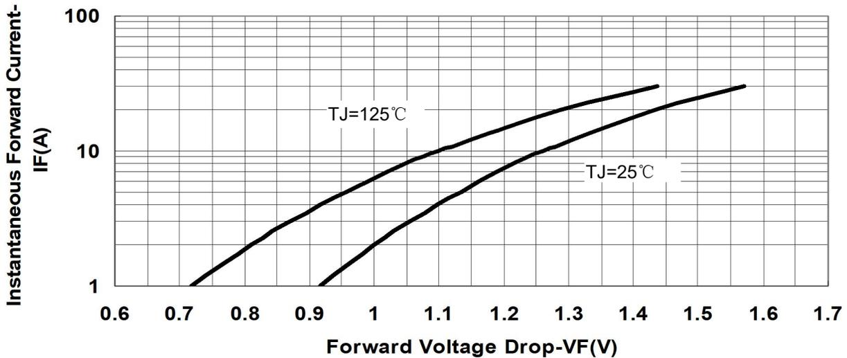
Fig.3-Typical Forward Voltage Drop Characteristics
