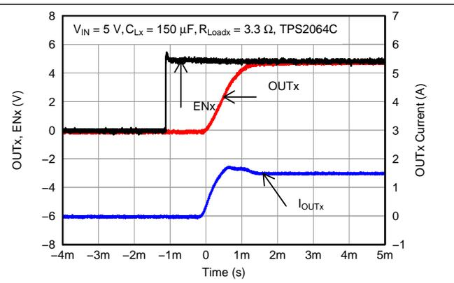
**Figure 14. TPS2064C Enable into 3.3 Ω and 150-μF Load**
