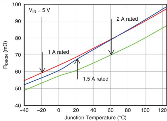
Figure 19. Input - output Resistance ( $R_{DS(ON)}$ ) vs Temperature
