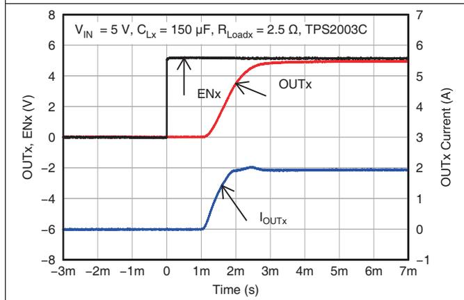
**Figure 17. TPS2003C Enable into 2.5 Ω and 150-μF Load**
