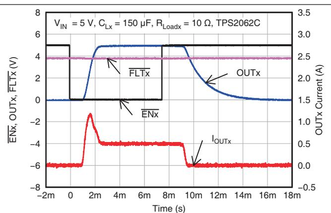
Figure 33. TPS2062C Enable/Disable into 10- $\Omega$  Load
