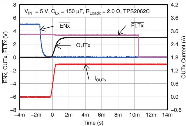
Figure 9. TPS2062C Enable With 2-Ω Load
