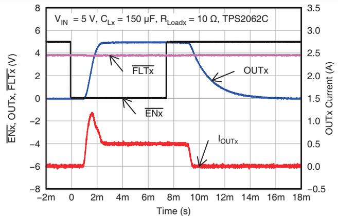
Figure 12. TPS2062C Enable and Disable into 10-Ω Load
