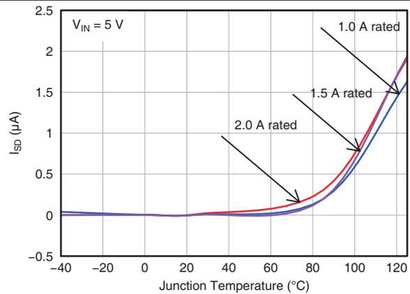
Figure 20. Supply Current (Device Disable) -  $I_{SD}$  vs Temperature
