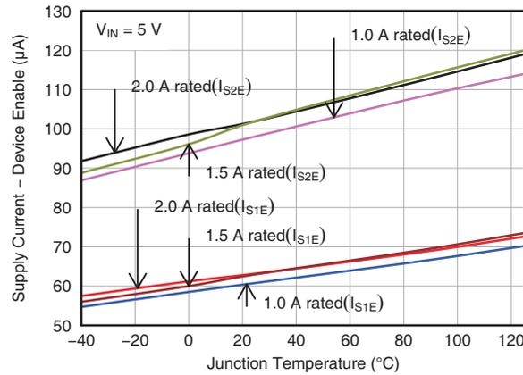
Figure 21. Supply Current (Enable) -  $I_{SE}$  vs Temperature
