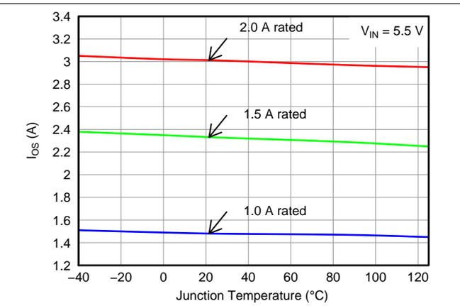
**Figure 18. Current Limit ( $I_{OS}$ ) vs Temperature**
