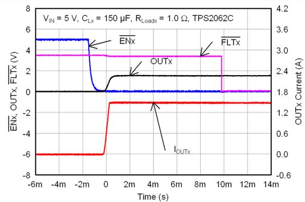
Figure 10. TPS2062C Enable With 1-Ω Load
