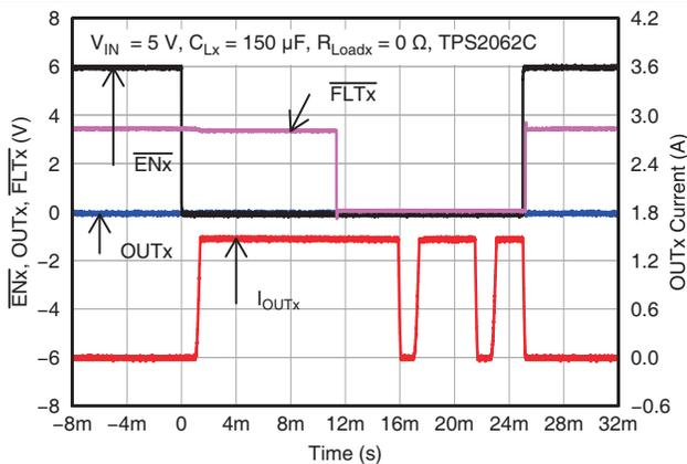
Figure 11. TPS2062C Enable and Disable into Output Short
