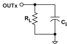
Figure 23. Output Rise / Fall Test Load
