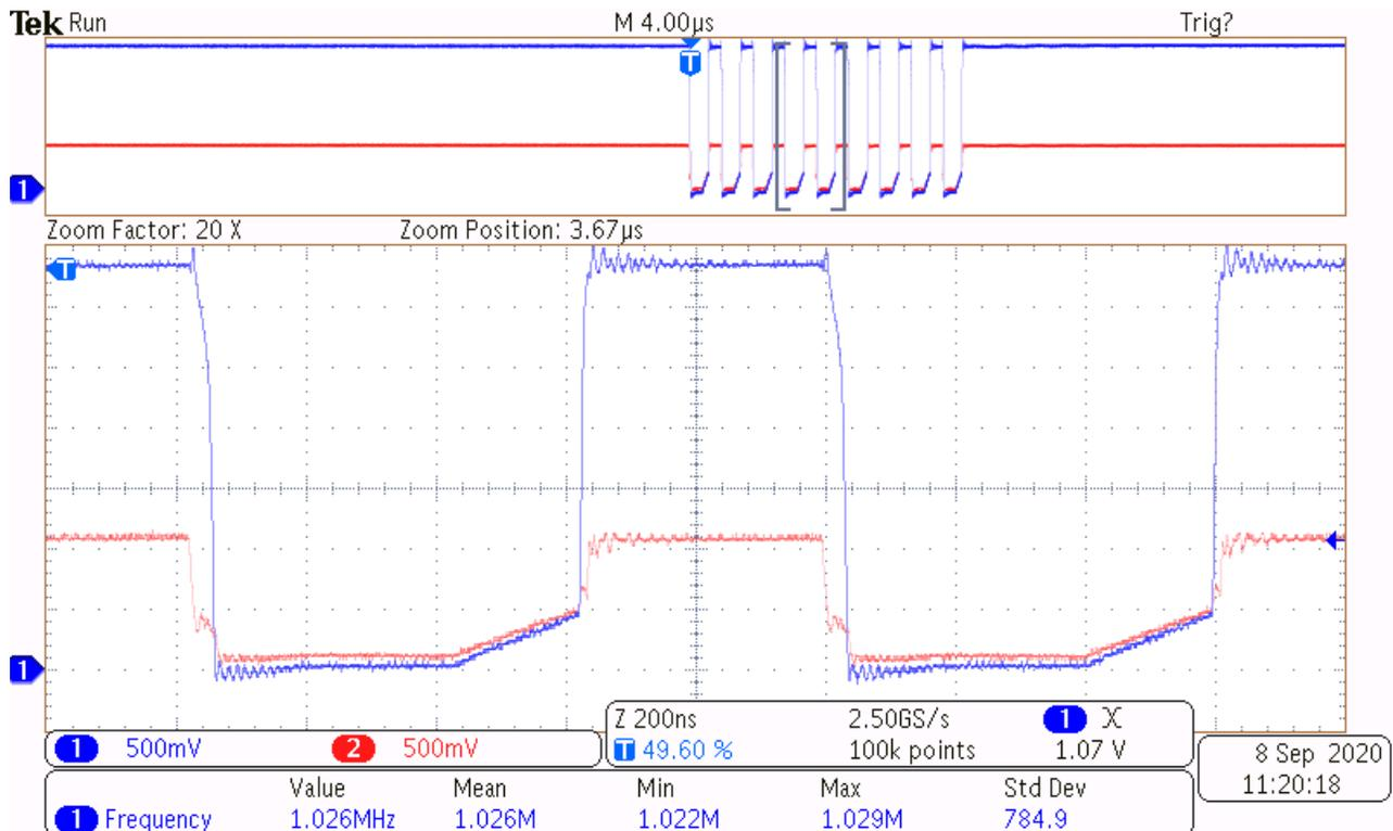
Figure 9-2. Level-Translation of a 1-MHz Signal
