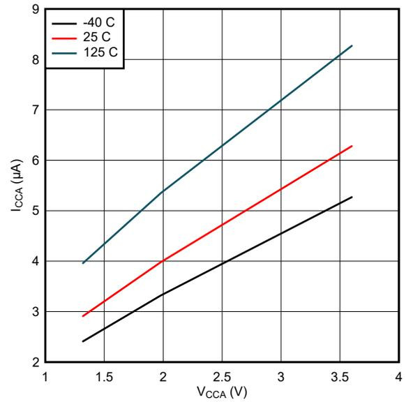
**Figure 6-2. I<sub>CCA</sub> (μA) vs V<sub>CCA</sub> (V)**
