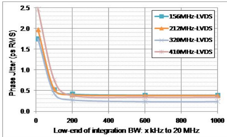
Figure 1. LVDS Phase Jitter (integrated phase noise)
