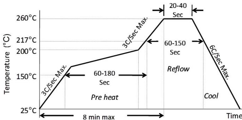
Figure 3. Solder Reflow Profile
