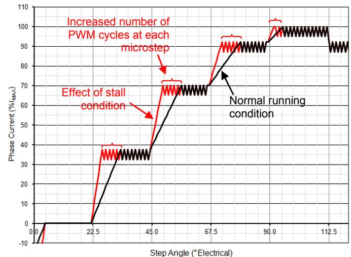
**Figure 5: Effect of Stall Condition on Current Rise**
