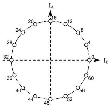
Figure 12: Quarter-step Phase Diagram Using STEP Input
