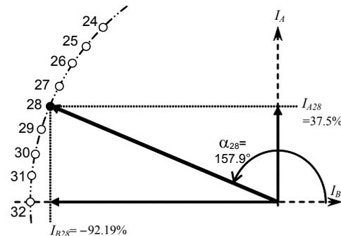
Figure 9: Calculation of Resultant Motor Current
