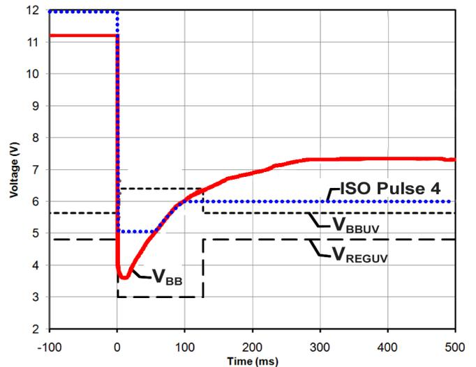
**Figure 3: A4980 Response to an Undervoltage Transient**
