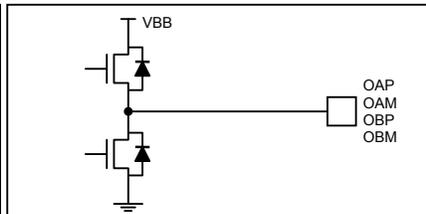
Figure 18i. Phase Outputs
