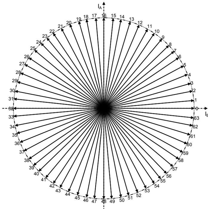
Figure 8. A4980 Phase Current Table as a Phase Diagram
