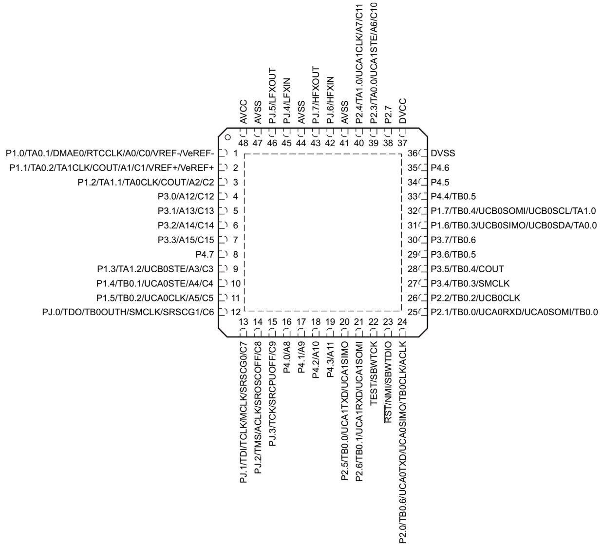
NOTE: TI recommends connecting the QFN package pad to  $V_{SS}$ .
