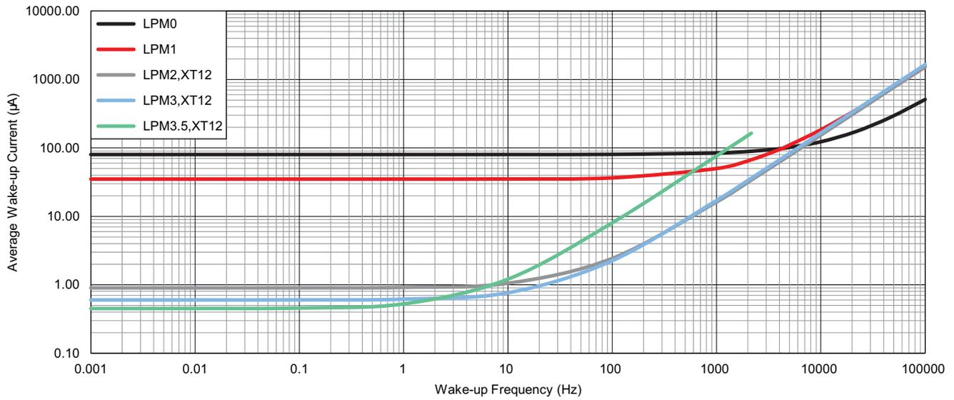
NOTE: The average wakeup current does not include the energy required in active mode; for example, for an interrupt service routine or to reconfigure the device.
