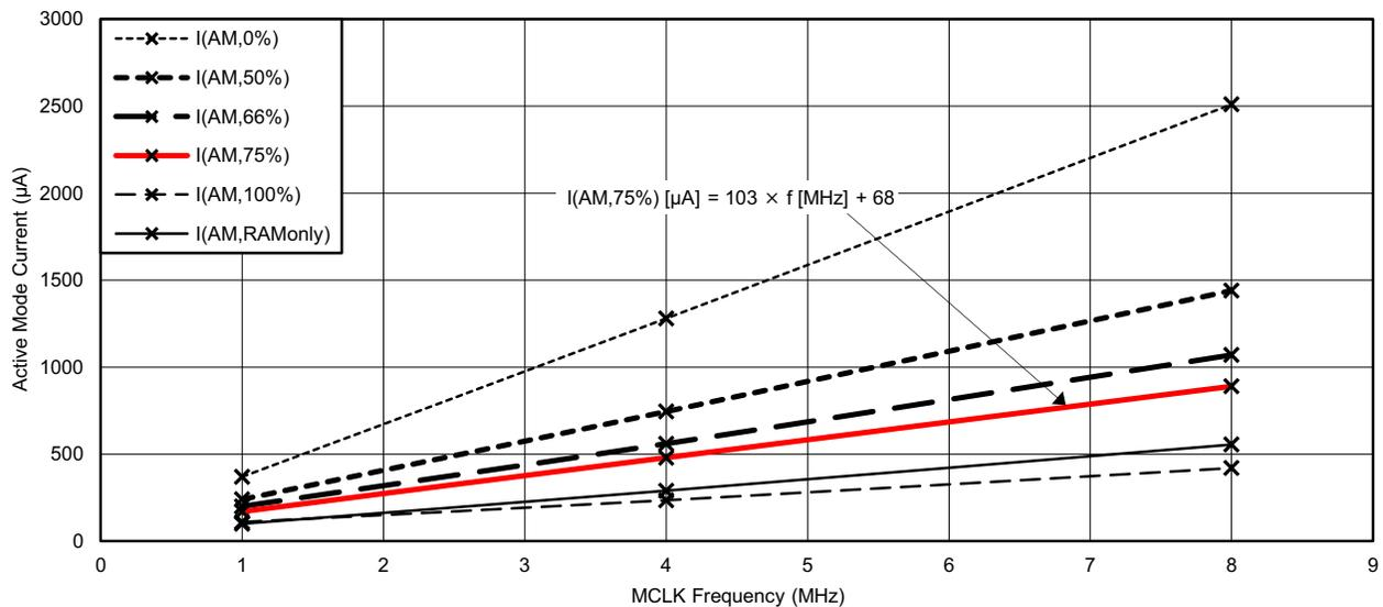
NOTE:  $I_{AM}$ , cache hit ratio): Program resides in FRAM. Data resides in SRAM. Average current dissipation varies with cache hit-to-miss ratio as specified. Cache hit ratio represents number cache accesses divided by the total number of FRAM accesses. For example, a 75% ratio implies three of every four accesses is from cache, and the remaining are FRAM accesses.
