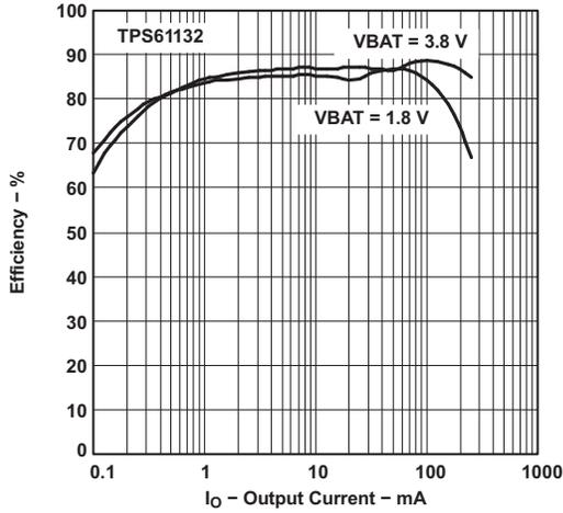
Figure 3. TPS61132 SEPIC Converter Efficiency vs Output Current
