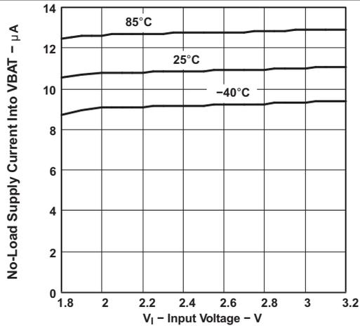
Figure 7. TPS61132 No-Load Supply Current Into VBAT vs Input Voltage
