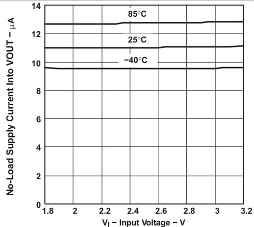
Figure 8. TPS61132 No-Load Supply Current Into VOUT vs Input Voltage
