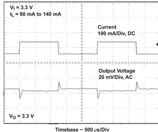
Figure 17. TPS61132 SEPIC Converter Load Transient Response
