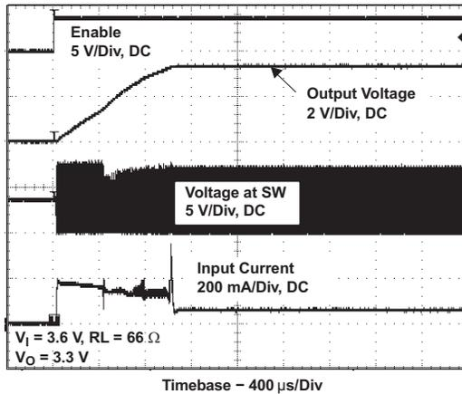
Figure 18. TPS61132 SEPIC Converter Start-Up After Enable
