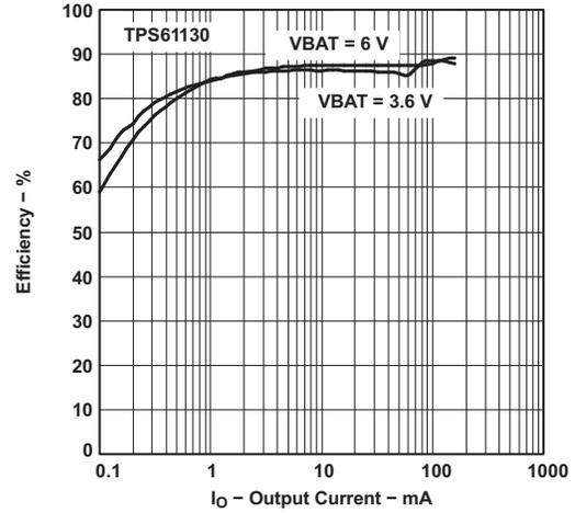
Figure 4. TPS61130 SEPIC Converter Efficiency vs Output Current
