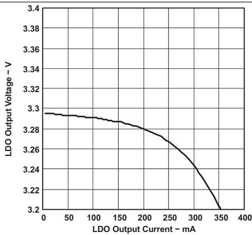
Figure 11. TPS61131 LDO Output Voltage vs LDO Output Current
