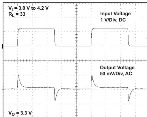
Figure 23. TPS61132 SEPIC Converter Line Transient Response
