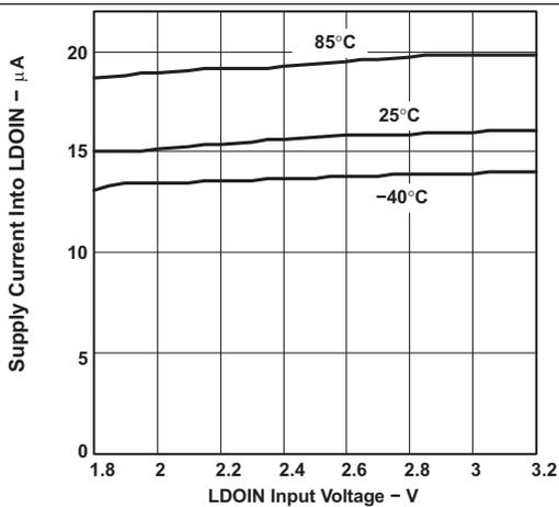
Figure 13. TPS61132 Supply Current Into LDOIN vs LDOIN Input Voltage
