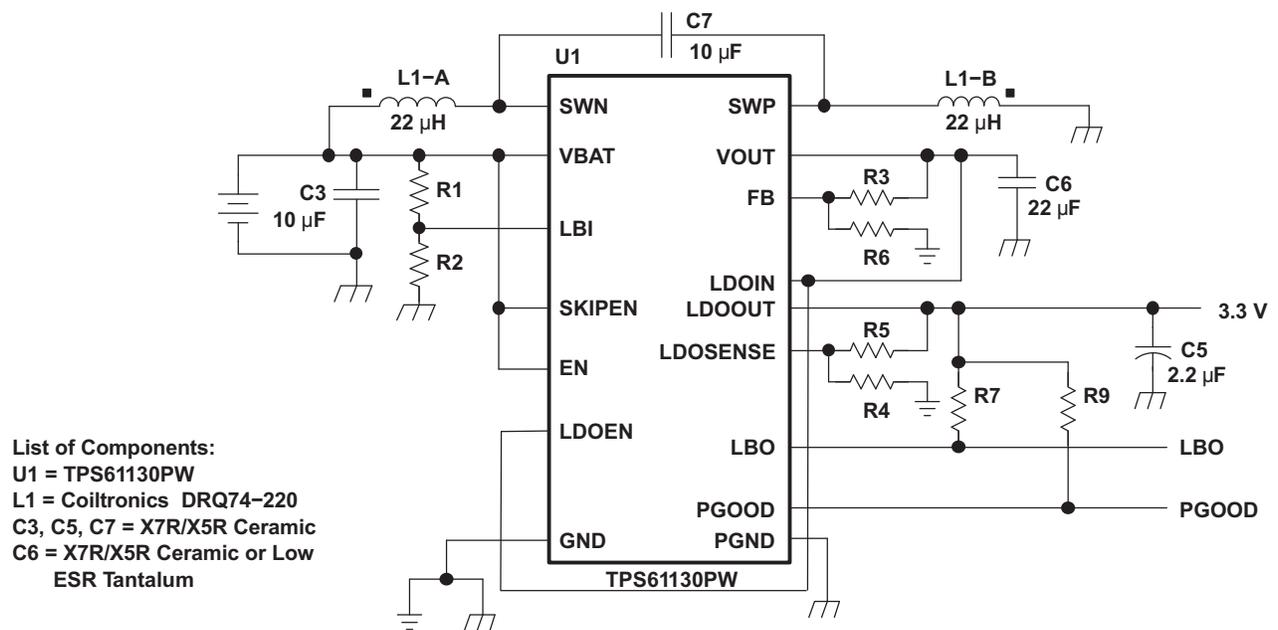
**Figure 26. Single Output Using LDO as Filter**
