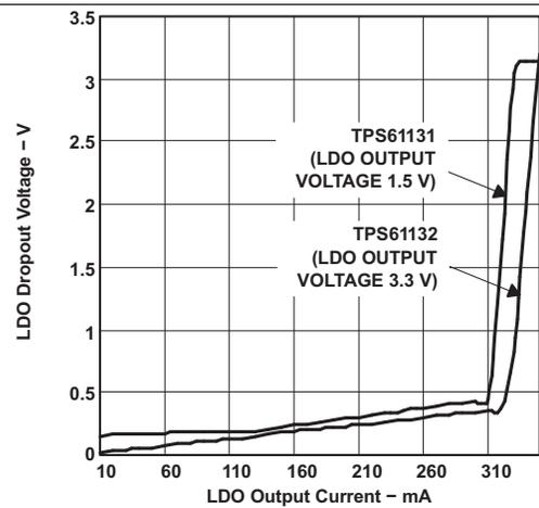
Figure 12. LDO Dropout Voltage vs LDO Output Current
