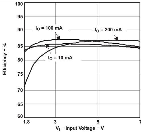
Figure 5. TPS61132 SEPIC Converter Efficiency vs Input Voltage
