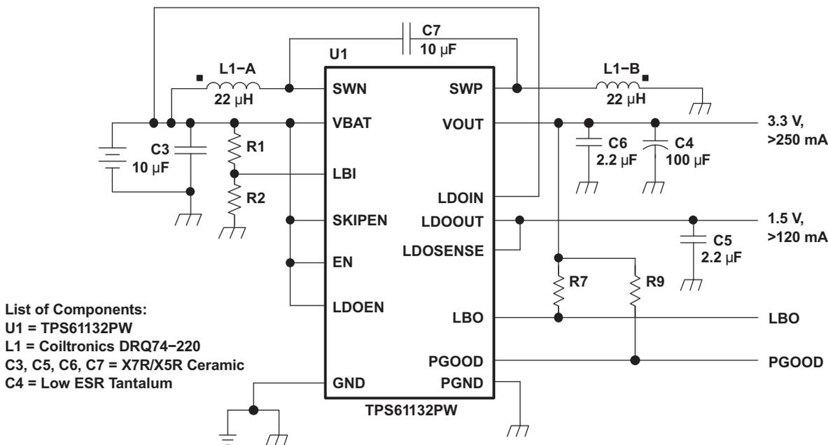
Figure 24. Solution for Maximum Output Power
