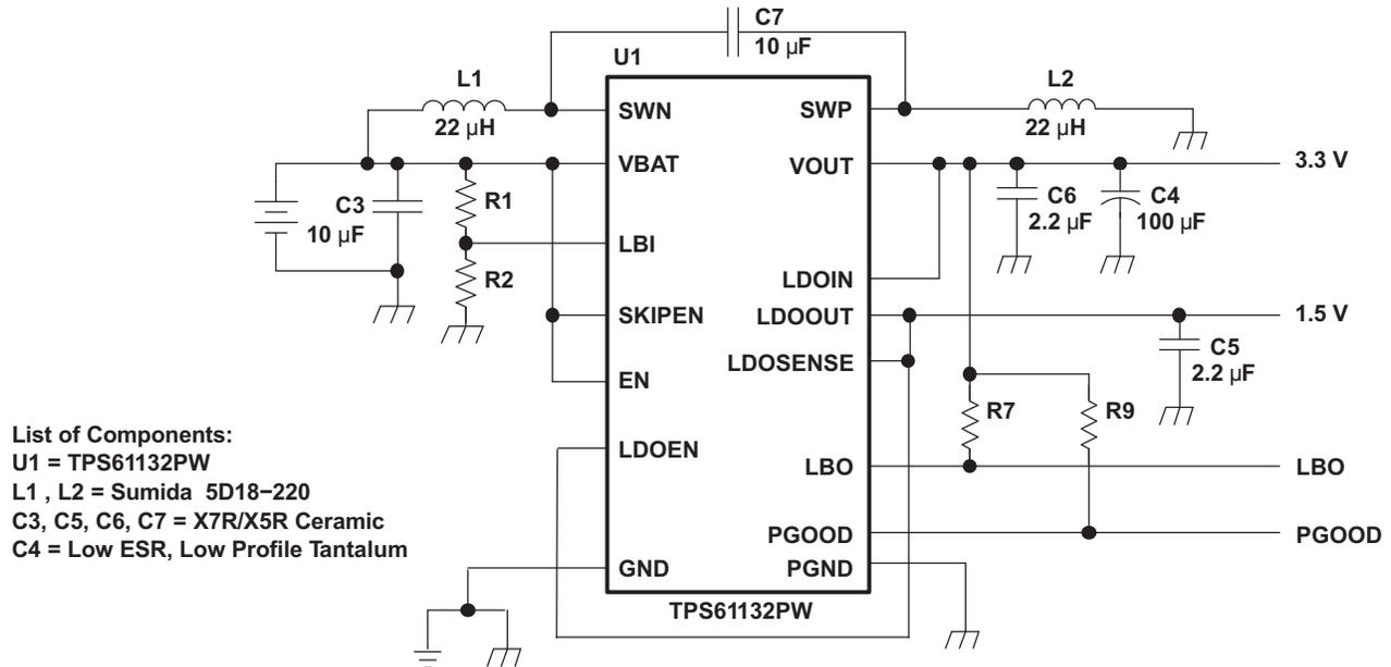
**Figure 25. Low Profile Solution, Maximum Height 1.8 mm**
