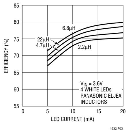
**Figure 3. Efficiency for Several Different Inductor Values**
