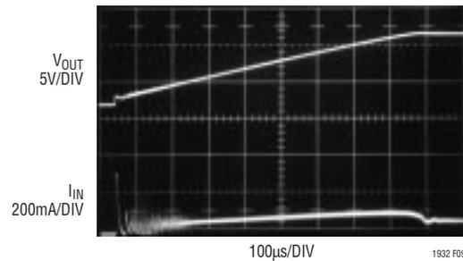
Figure 9. Input Current at Start-Up with Soft-Start
