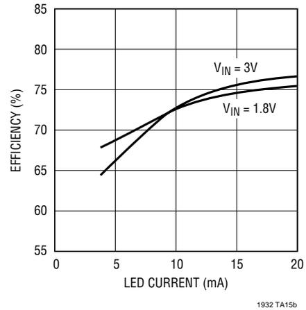
2-Cell Driver for Three White LEDs
