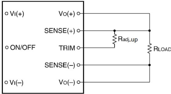
Figure 12. Circuit Configuration to Increase Output Voltage.
