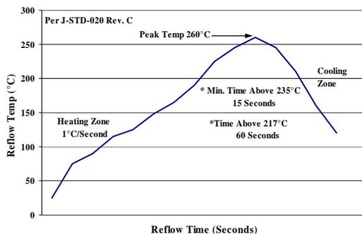
Figure 22. Recommended linear reflow profile using Sn/Ag/Cu solder.
