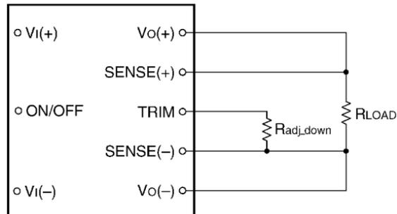
**Figure 11. Circuit Configuration to Decrease Output Voltage.**
