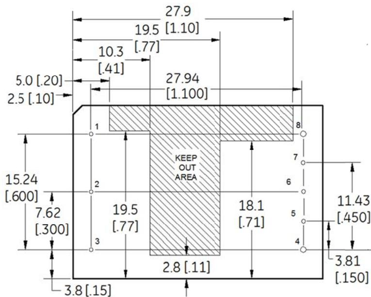
For .025 x .030 rectangular pin, use a .050 diameter plated through hole
