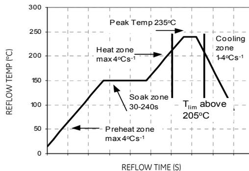
Figure 20. Recommended Reflow Profile for Sn/Pb solder.
