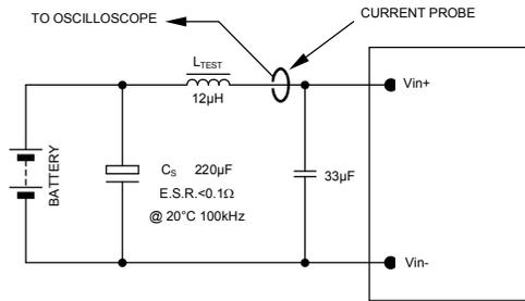
NOTE: Measure input reflected ripple current with a simulated source inductance ( $L_{TEST}$ ) of 12µH. Capacitor  $C_S$  offsets possible battery impedance. Measure current as shown above.
