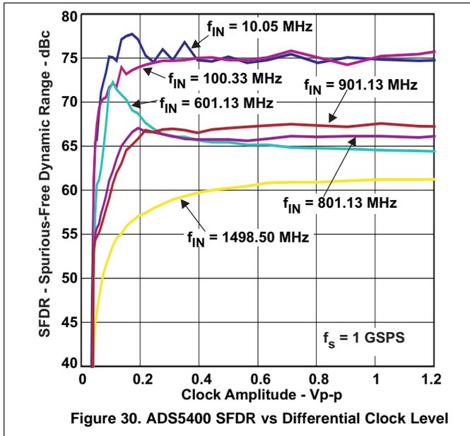
Figure 30. ADS5400 SFDR vs Differential Clock Level
