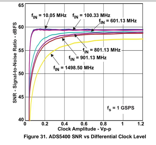
Figure 31. ADS5400 SNR vs Differential Clock Level
