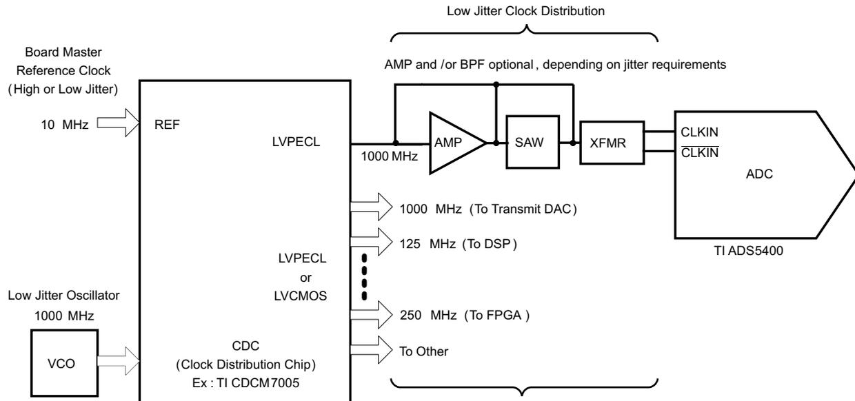
This is a general block diagram example: Consult the datasheet of the CDCM7005 for proper schematic and for specifications regarding allowable input and output frequency and amplitude ranges.
