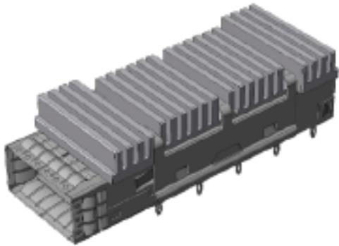
The interconnect system comprises a 38 position 0.8mm pitch connector and a press-fit cage designed to comply with the Quad Small Form-factor Pluggable (QSFP) Transceiver Specifications.
