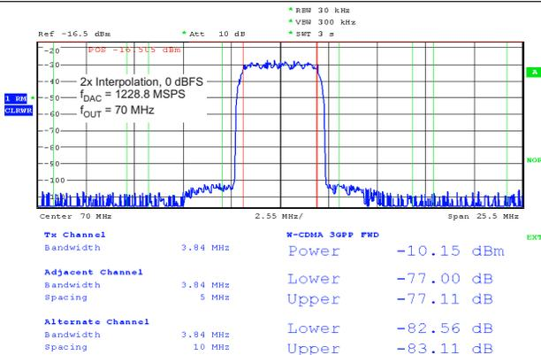
Figure 27. Single Carrier W-CDMA Test Model 1
