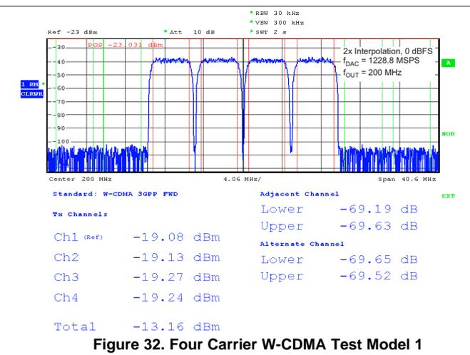
Figure 32. Four Carrier W-CDMA Test Model 1
