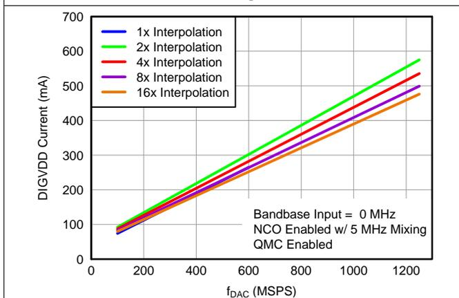
**Figure 41. DIGVDD Current vs  $f_{DAC}$  Over Interpolation**
