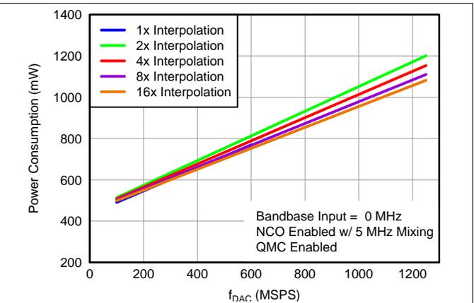
**Figure 38. Power Consumption vs  $f_{DAC}$  Over Interpolation**
