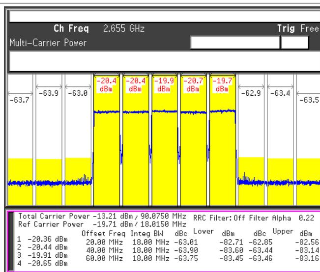
DAC Output IF = 0 MHz, LO = 2655 MHz, DAC Clock = External Clock Source from LMK04806
