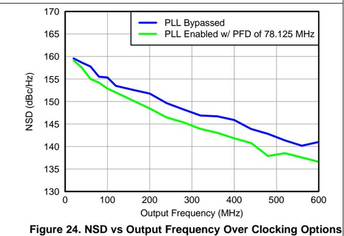
Figure 24. NSD vs Output Frequency Over Clocking Options
