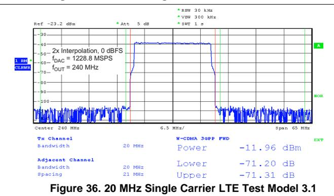
Figure 36. 20 MHz Single Carrier LTE Test Model 3.1
