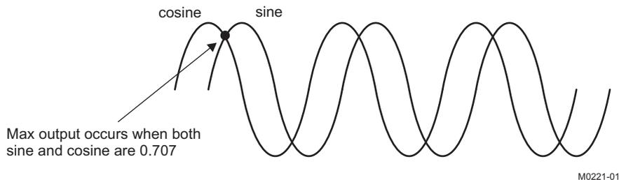
**Figure 70. Maximum Output of the Complex Signal Multiplier**
