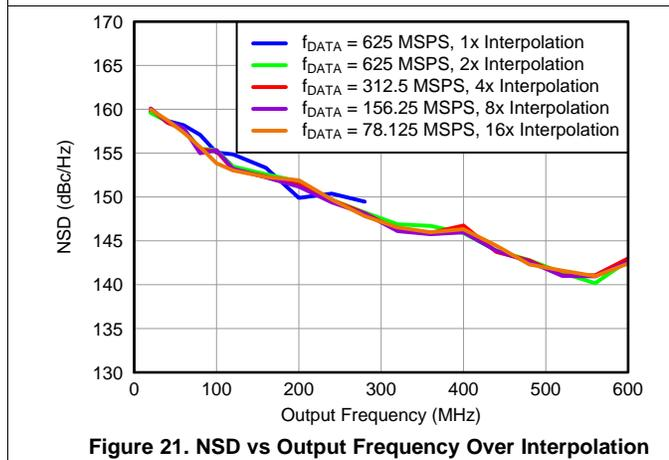
Figure 21. NSD vs Output Frequency Over Interpolation
