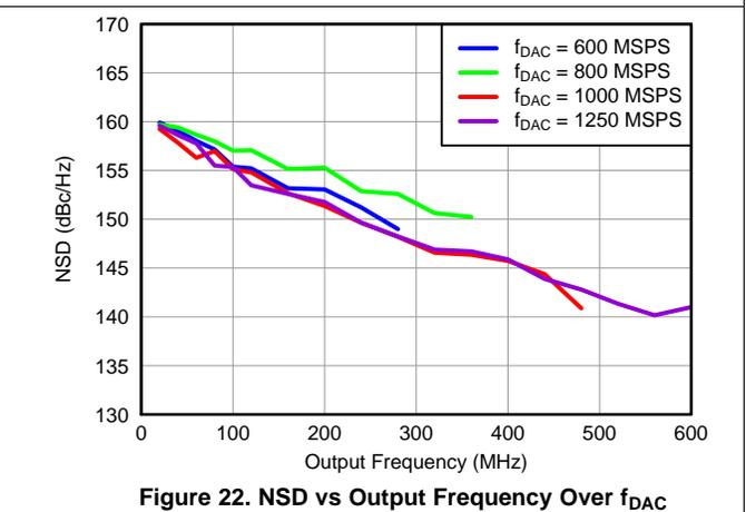
Figure 22. NSD vs Output Frequency Over  $f_{DAC}$
