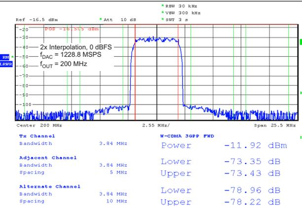
Figure 29. Single Carrier W-CDMA Test Model 1
