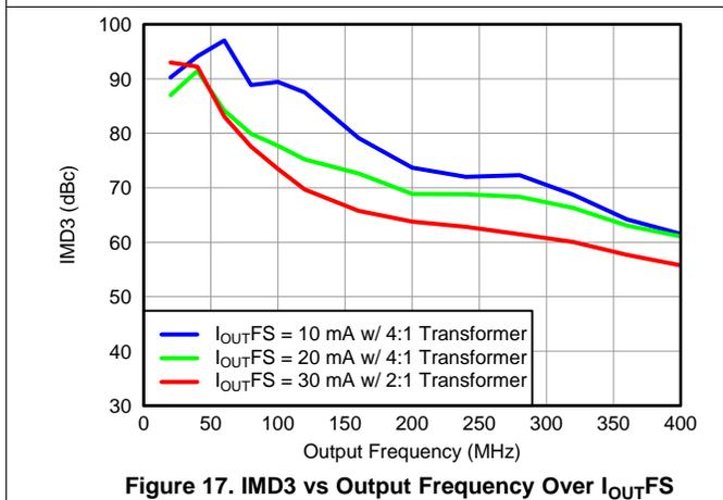
**Figure 17. IMD3 vs Output Frequency Over  $I_{OUTFS}$**
