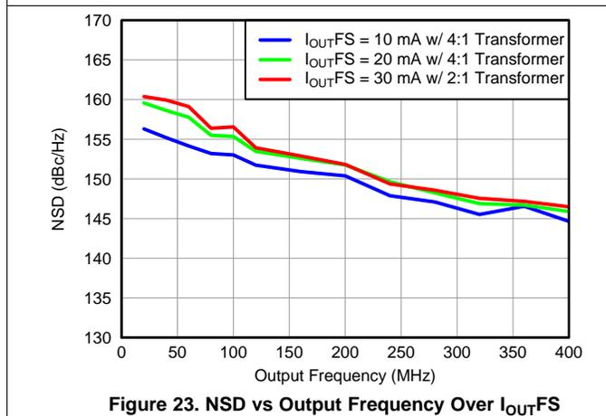
Figure 23. NSD vs Output Frequency Over  $I_{OUTFS}$
