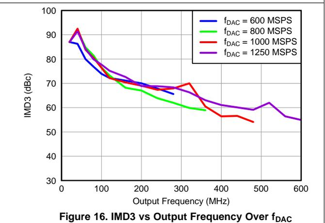
**Figure 16. IMD3 vs Output Frequency Over  $f_{DAC}$**
