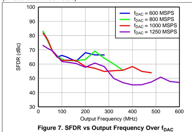
Figure 7. SFDR vs Output Frequency Over  $f_{DAC}$
