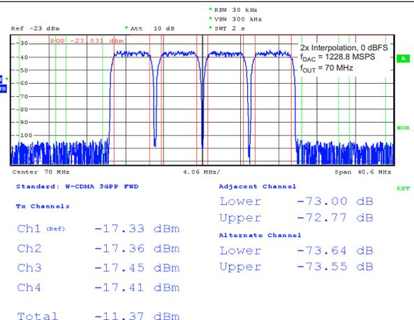
Figure 30. Four Carrier W-CDMA Test Model 1
