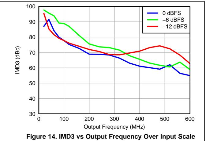
**Figure 14. IMD3 vs Output Frequency Over Input Scale**
