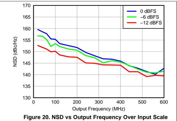
Figure 20. NSD vs Output Frequency Over Input Scale
