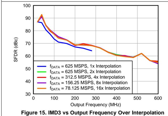
**Figure 15. IMD3 vs Output Frequency Over Interpolation**
