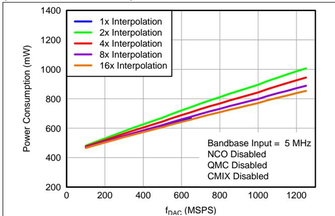
**Figure 37. Power Consumption vs  $f_{DAC}$  Over Interpolation**
