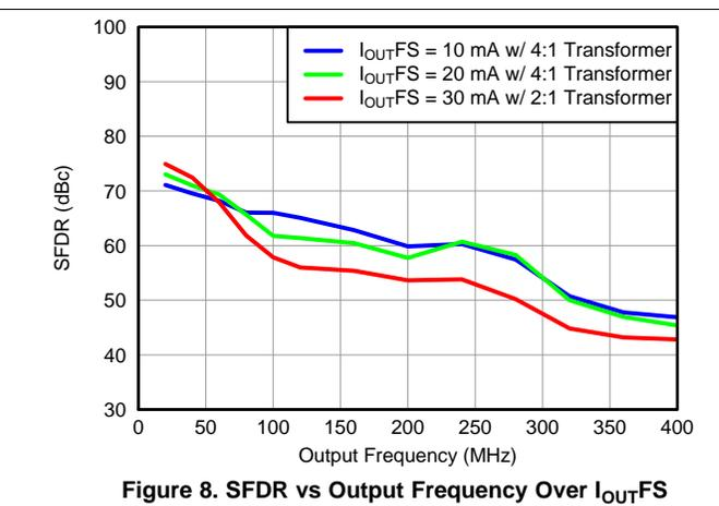
Figure 8. SFDR vs Output Frequency Over  $I_{OUTFS}$
