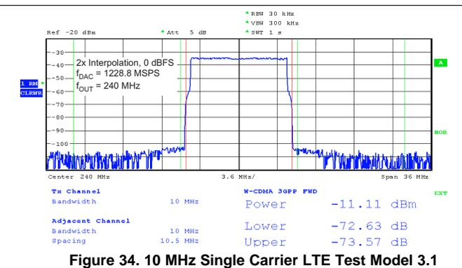
Figure 34. 10 MHz Single Carrier LTE Test Model 3.1
