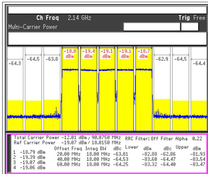
DAC Output IF = 0 MHz, LO = 2140 MHz, DAC Clock = External Clock Source from LMK04806
