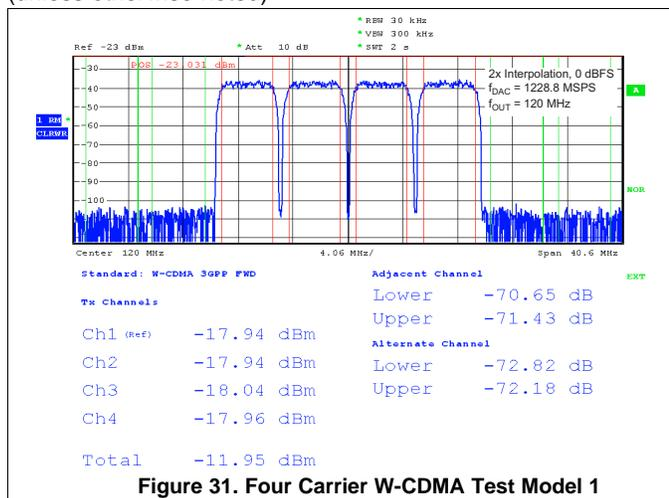
Figure 31. Four Carrier W-CDMA Test Model 1
