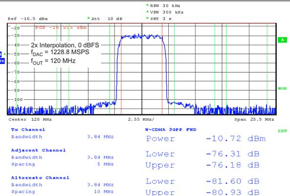
Figure 28. Single Carrier W-CDMA Test Model 1
