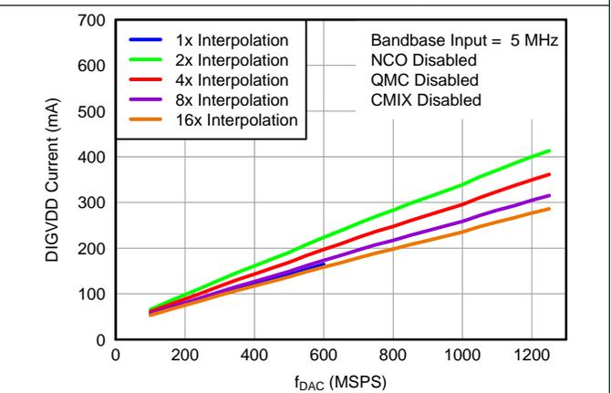
**Figure 40. DIGVDD Current vs  $f_{DAC}$  Over Interpolation**
