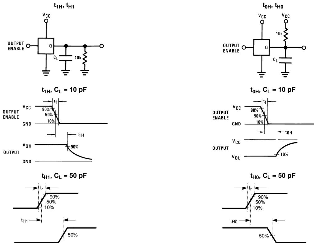
Figure 10. TRI-STATE Test Circuits and Timing Diagrams
