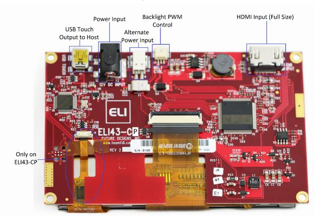
Power may be supplied either via the 2-pin terminal block J8 or via the 2.1mm power jack P2 (center positive)
