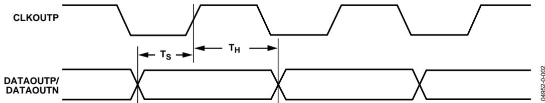
Figure 2. Output Timing
