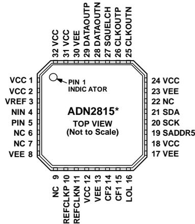
\*THERE IS AN EXPOSED PAD ON THE BOTTOM OF THE PACKAGE THAT MUST BE CONNECTED TO GND.
