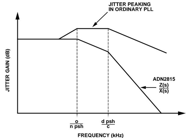
Figure 14. ADN2815 Jitter Response vs. Conventional PLL
