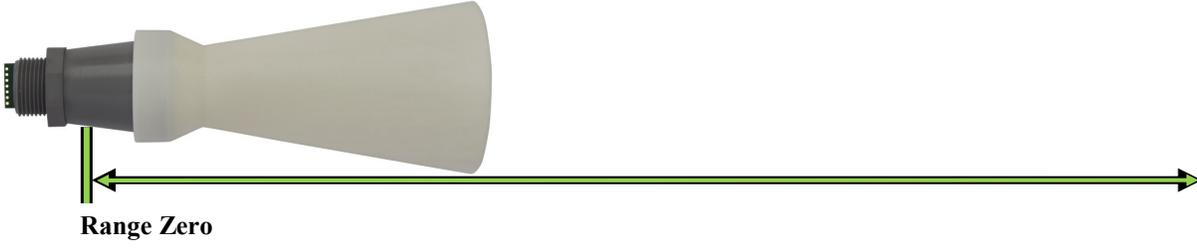
The range is measured from the front of the transducer to the target.
