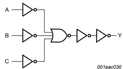
Fig. 3. Logic diagram
