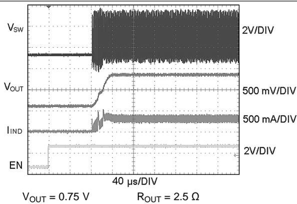
Figure 39. Start-Up Into PWM Mode
