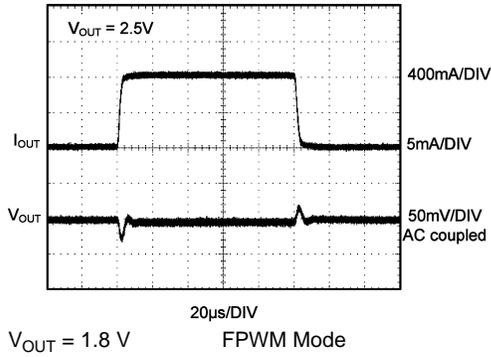
Figure 49. Load Transient Response
