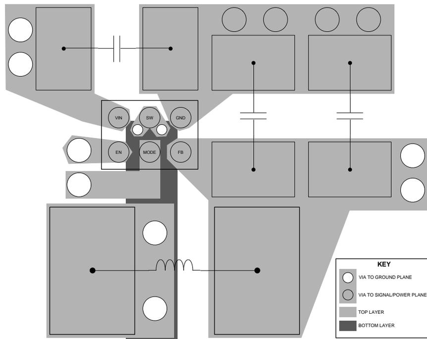
**Figure 53. LM3291 Layout Example**
