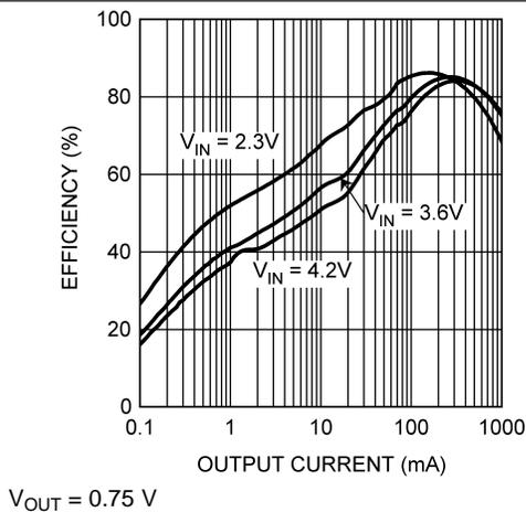
Figure 11. Efficiency vs, Output Current, ECO Mode
