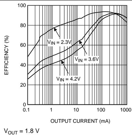
Figure 12. Efficiency vs Output Current, ECO Mode
