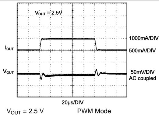
Figure 37. Load Transient Reponse
