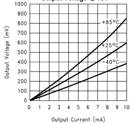
**Output Sinking Current vs. Output Voltage @ 15V**
