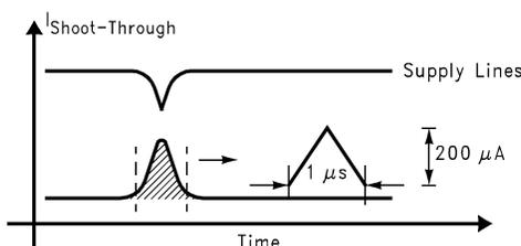
$$\text{Area of } \Delta = \frac{1}{2} (1 \mu\text{s} \times 200 \mu\text{A}) = 100 \text{ pC}$$
