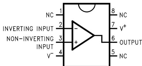
**Figure 1. 8-Pin SOIC-8
