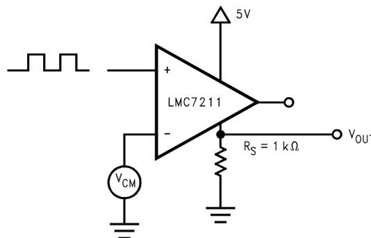
**Figure 4. Circuit for Measurement of the Shoot-Through Current**
