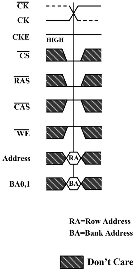
**Figure 6. t<sub>RCD</sub> and t<sub>RRD</sub> Definition**
