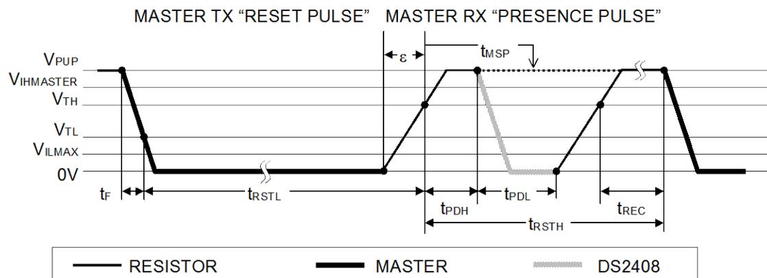
After the bus master has released the line it goes into receive mode (RX). The 1-Wire bus is then pulled to  $V_{PUP}$  via the pullup resistor or, in case of a DS2480B driver, by active circuitry. When the  $V_{TH}$  threshold is crossed, the DS2408 waits for  $t_{PDH}$  and then transmits a Presence Pulse by pulling the line low for  $t_{PDL}$ . To detect a presence pulse, the master must test the logical state of the 1-Wire line at  $t_{MSP}$ .
