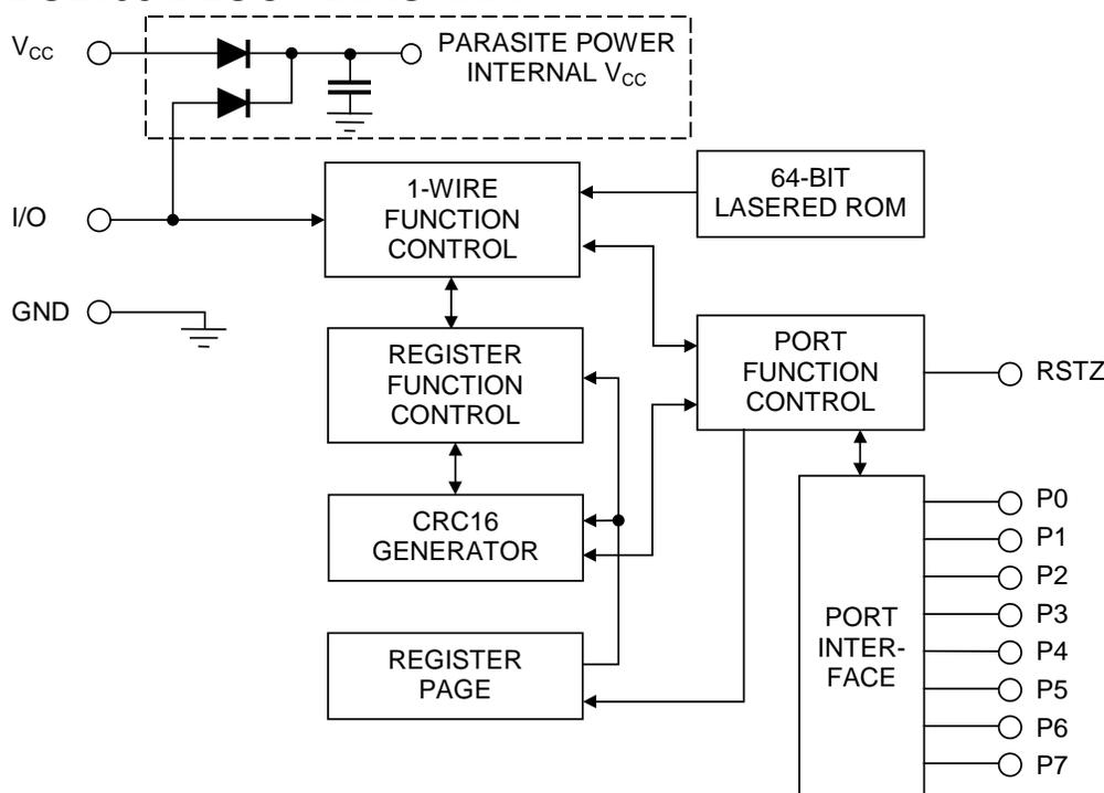
**Figure 2. HIERARCHICAL STRUCTURE FOR 1-Wire PROTOCOL**
