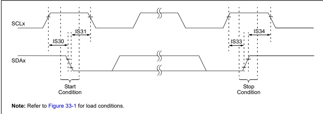
**FIGURE 33-17: I2Cx BUS DATA TIMING CHARACTERISTICS (SLAVE MODE)**
