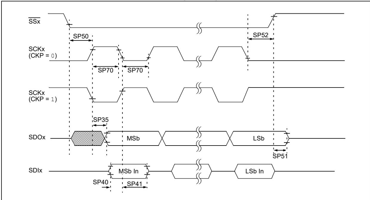
**FIGURE 33-13: SPIx MODULE SLAVE MODE (CKE = 1) TIMING CHARACTERISTICS**
