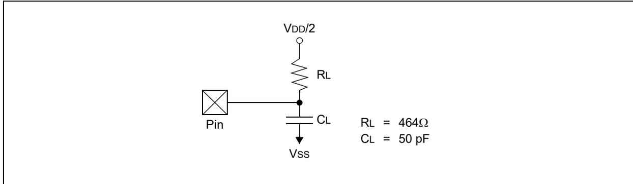
**FIGURE 33-2: CLKO AND I/O TIMING CHARACTERISTICS**
