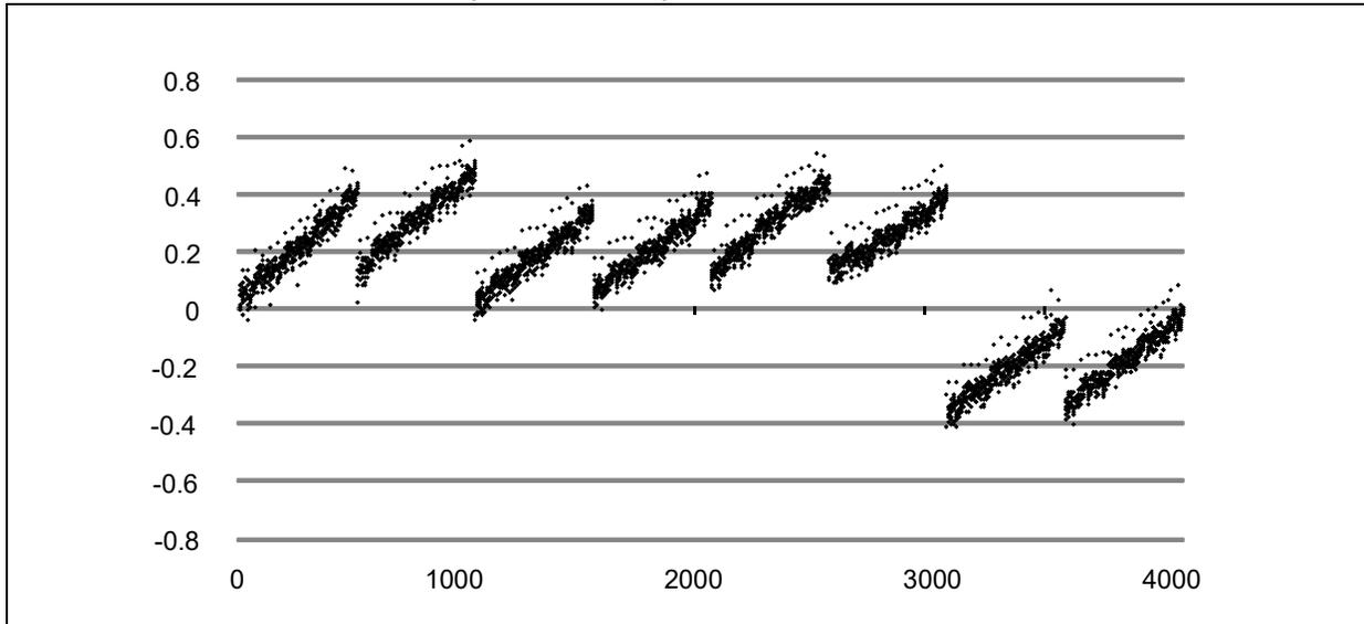
FIGURE 33-21: DNL vs. CODE (12-BIT MODE)<sup>(1)</sup>
