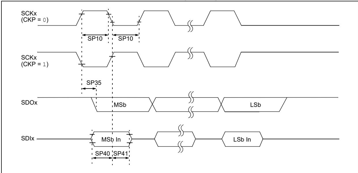
**FIGURE 33-11: SPIx MODULE MASTER MODE (CKE = 1) TIMING CHARACTERISTICS**
