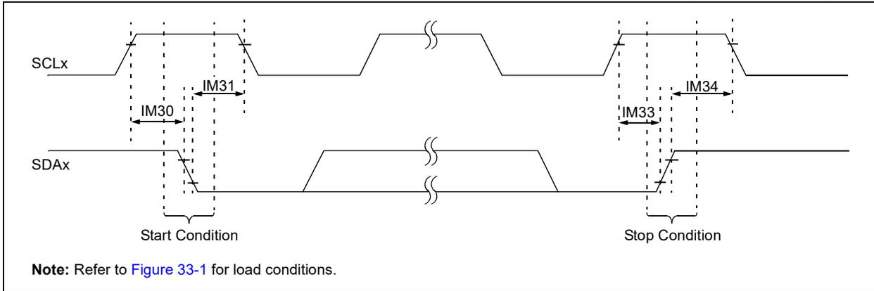
**FIGURE 33-15: I2Cx BUS DATA TIMING CHARACTERISTICS (MASTER MODE)**
