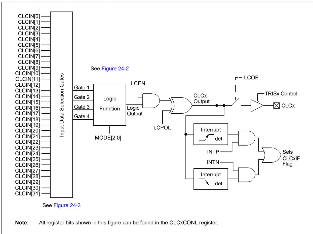
**Note:** All register bits shown in this figure can be found in the CLCxCONL register.
