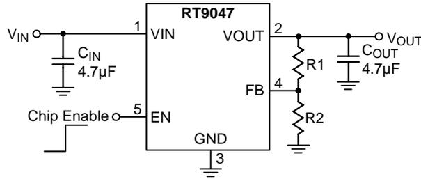
$$V_{OUT} = V_{FB} \times \left(1 + \frac{R1}{R2}\right) \text{ Volts}$$
