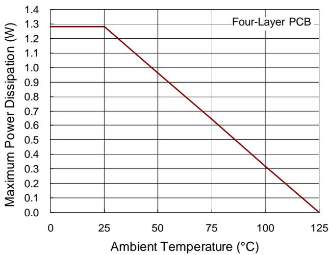
Figure 2. Derating Curves for the RT9047 Package
