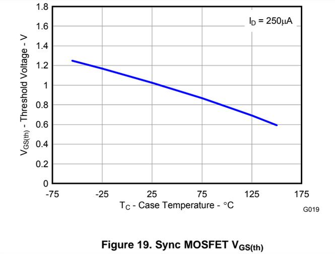
Figure 19. Sync MOSFET V<sub>GS(th)</sub>
