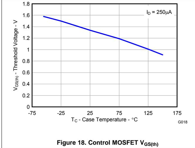
Figure 18. Control MOSFET V<sub>GS(th)</sub>
