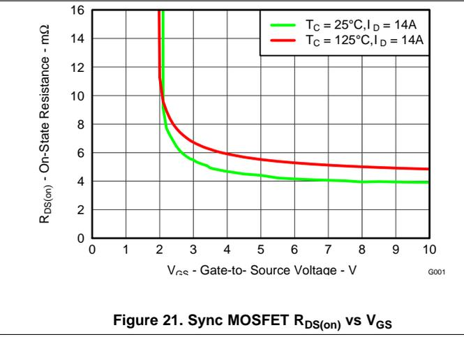
Figure 21. Sync MOSFET R<sub>DS(on)</sub> vs V<sub>GS</sub>
