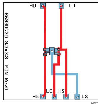
$\text{Max } R_{\theta JA} = 140^\circ\text{C/W}$
