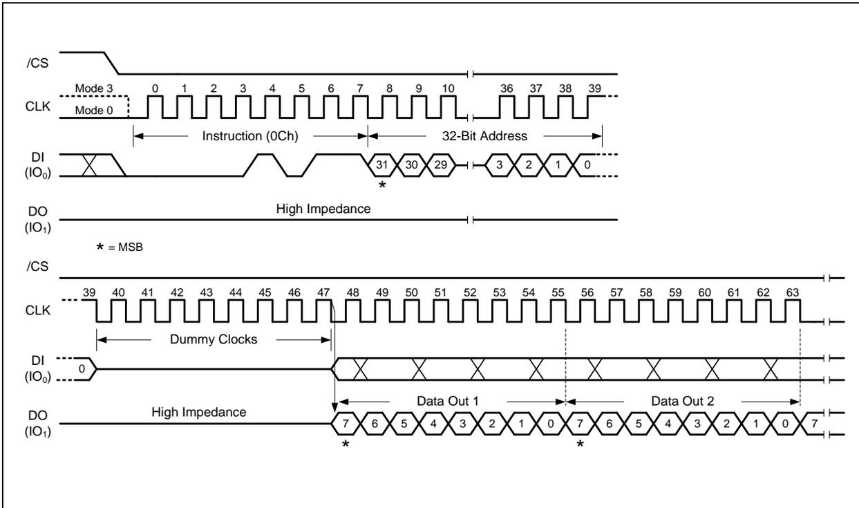
Figure 17. Fast Read with 4-Byte Address Instruction
