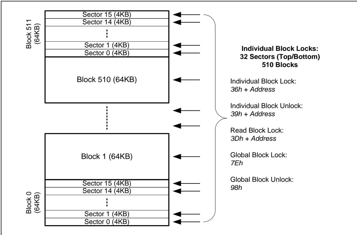
Figure 3d. Individual Block/Sector Locks (Single Die W25Q256JW-IQ)
