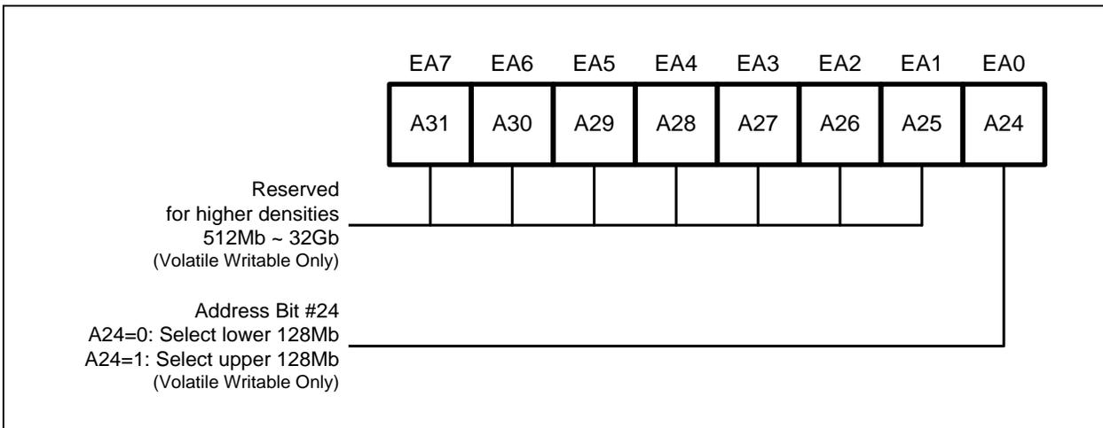
Figure 3e. Extended Address Register (Single Die W25Q256JW-IQ)
