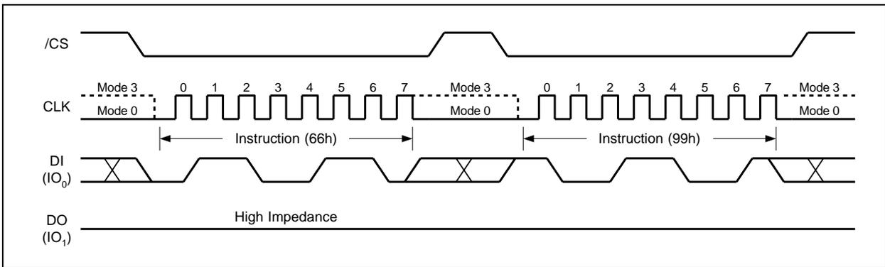
Figure 57. Enable Reset and Reset Instruction Sequence
