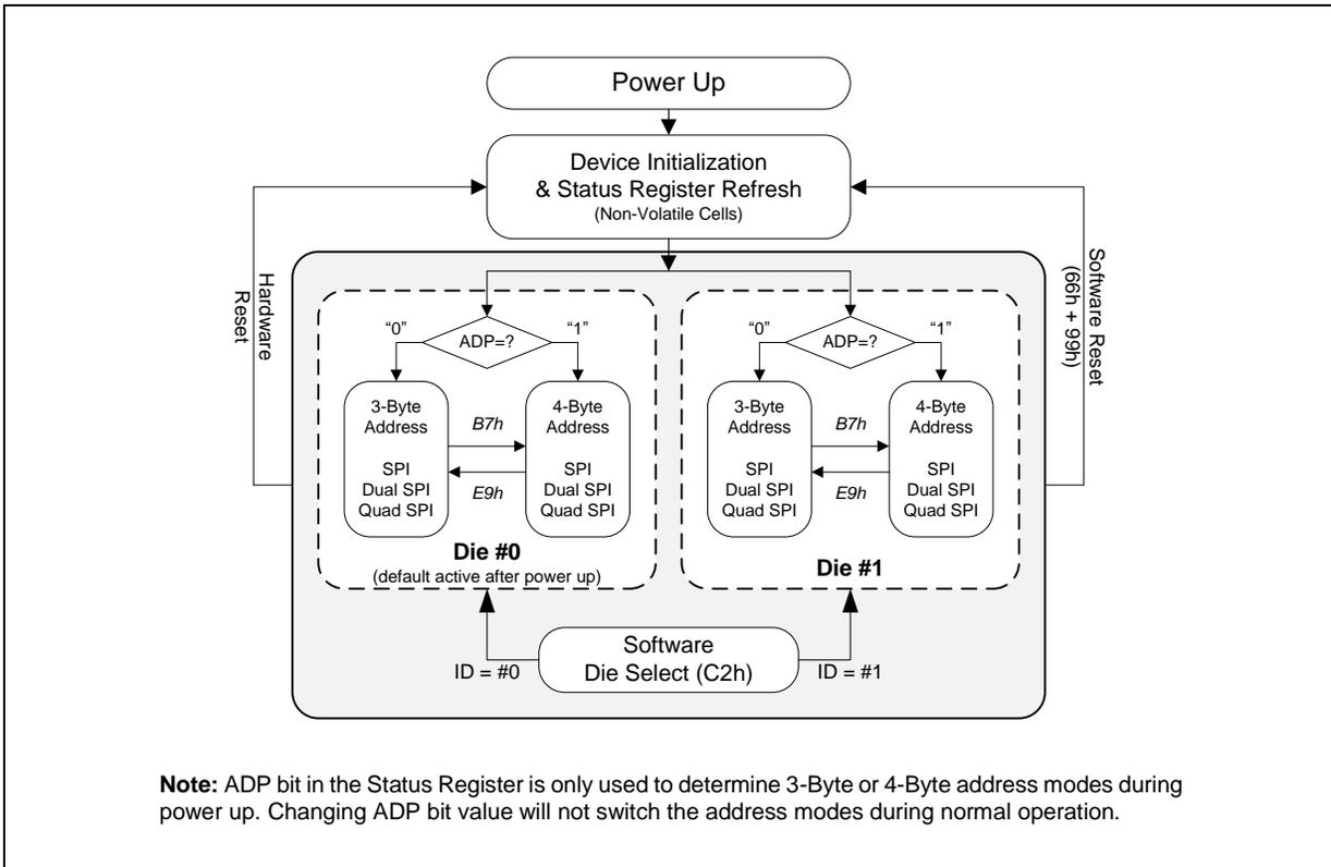
Figure 2c. W25M512JW-IQ Serial Flash Memory Operation Diagram
