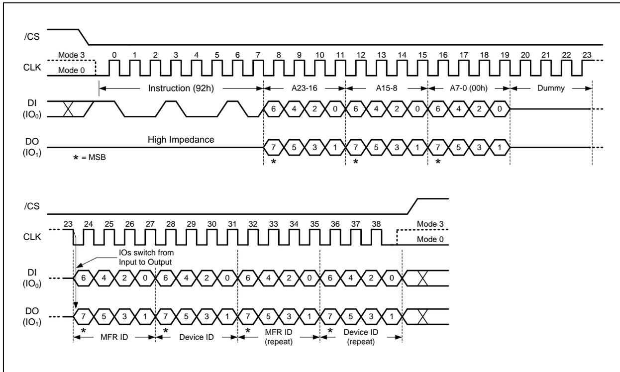
Figure 44. Read Manufacturer / Device ID Dual I/O Instruction
