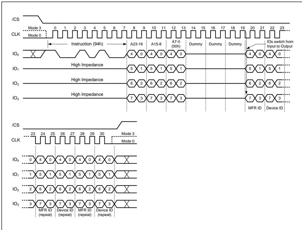
Figure 45. Read Manufacturer / Device ID Quad I/O Instruction
