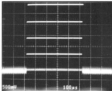
Figure 17.  $V_{LOG}$  Response to a 10.7 MHz CW Signal Modulated by a 25  $\mu$ s Wide Pulse with a 25 kHz Repetition Rate Using 200 pF Input Coupling Capacitors. The Input Signal Goes from +5 dBm to -75 dBm in 20 dB Steps.
