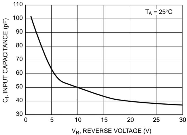
Figure 3. Input Capacitance
