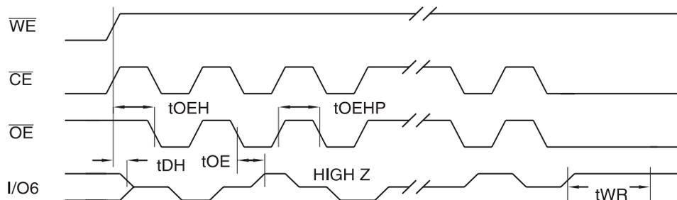
Notes: 1. Toggling either  $\overline{OE}$  or  $\overline{CE}$  or both  $\overline{OE}$  and  $\overline{CE}$  will operate toggle bit. The  $t_{OEHP}$  specification must be met by the toggling input(s).
