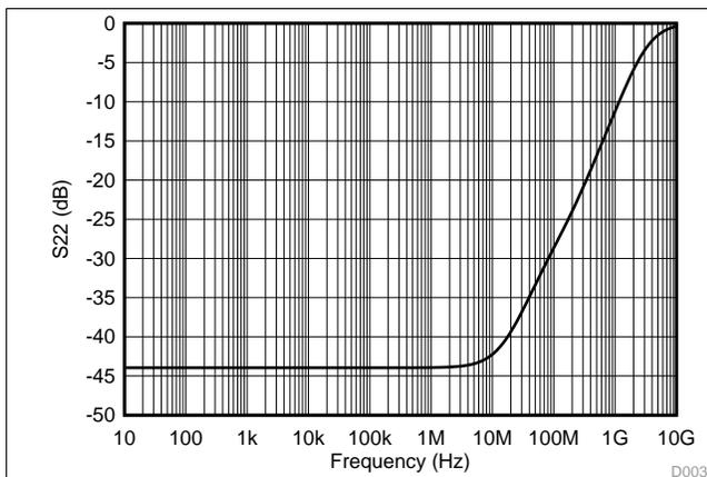
Figure 4. Return Loss ( $R_L$ ), Transmitter
