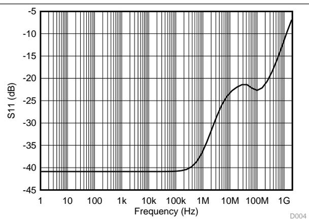
Figure 5. Return Loss ( $R_L$ ), Receiver
