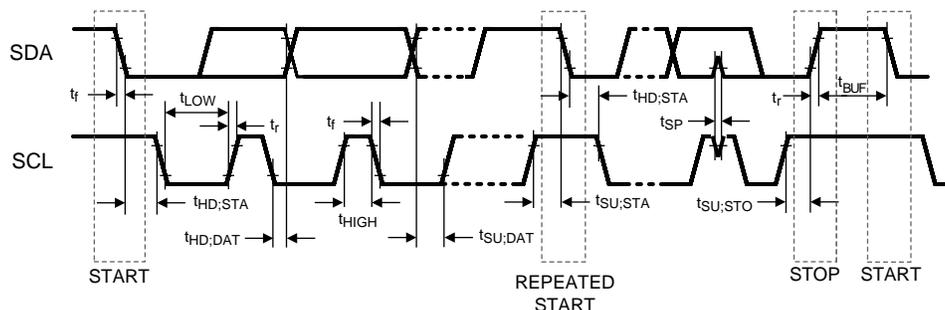
**Figure 1. I<sup>2</sup>C Timing**
