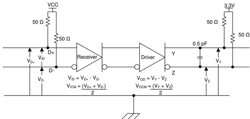
Figure 7-2. TMSD Main Link Test Circuit
