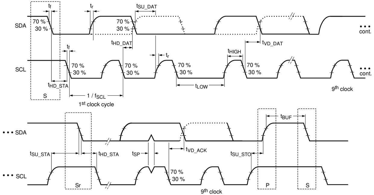
Figure 7-9. I<sup>2</sup>C SCL and SDA Timing
