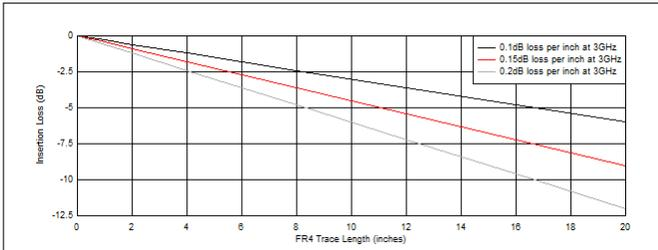
**Figure 9-3. FR4 Trace Insertion Loss at 3 GHz**
