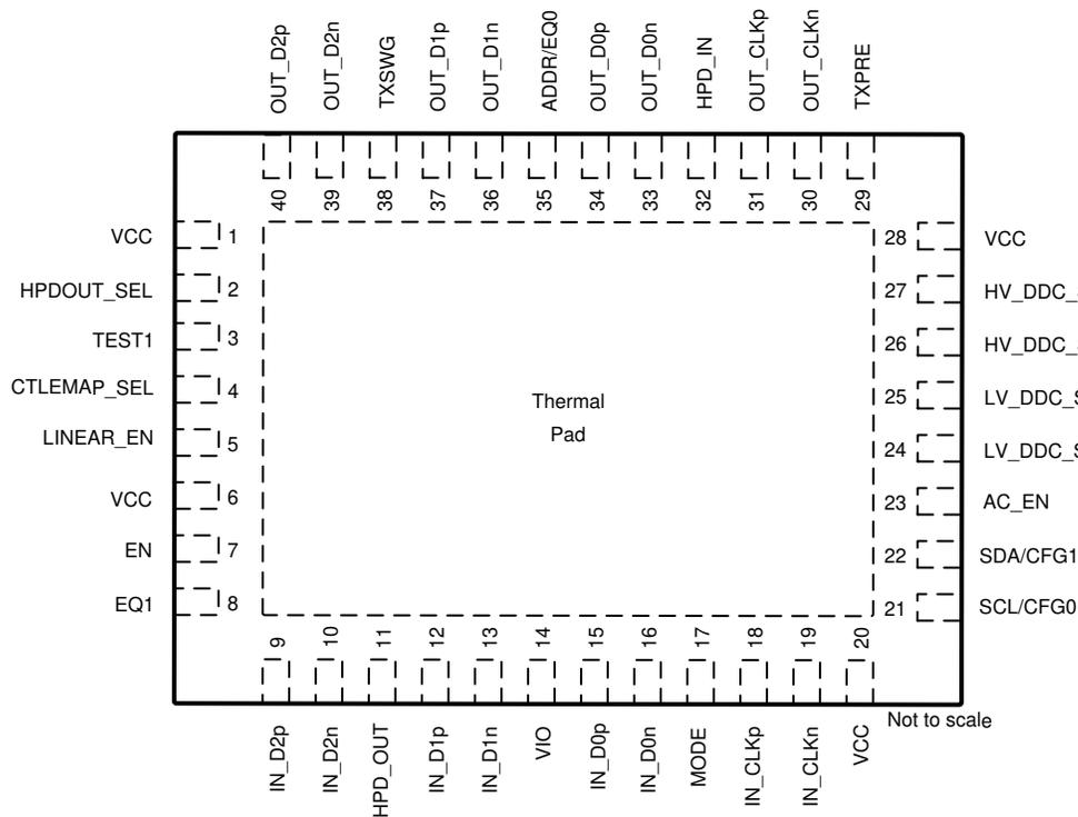
Figure 5-1. RNQ Package, 40-Pin WQFN (Top View)
