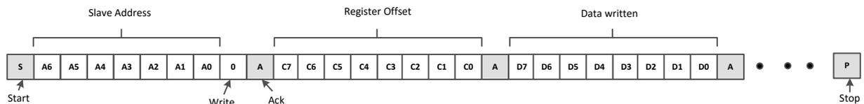
Figure 8-11. I<sup>2</sup>C Write with Data
