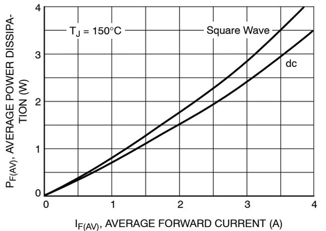
Figure 8. Typical Forward Power Dissipation
