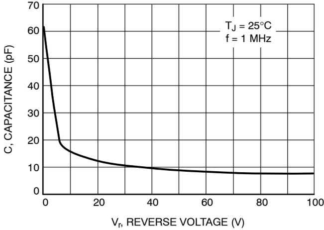
Figure 5. Typical Capacitance
