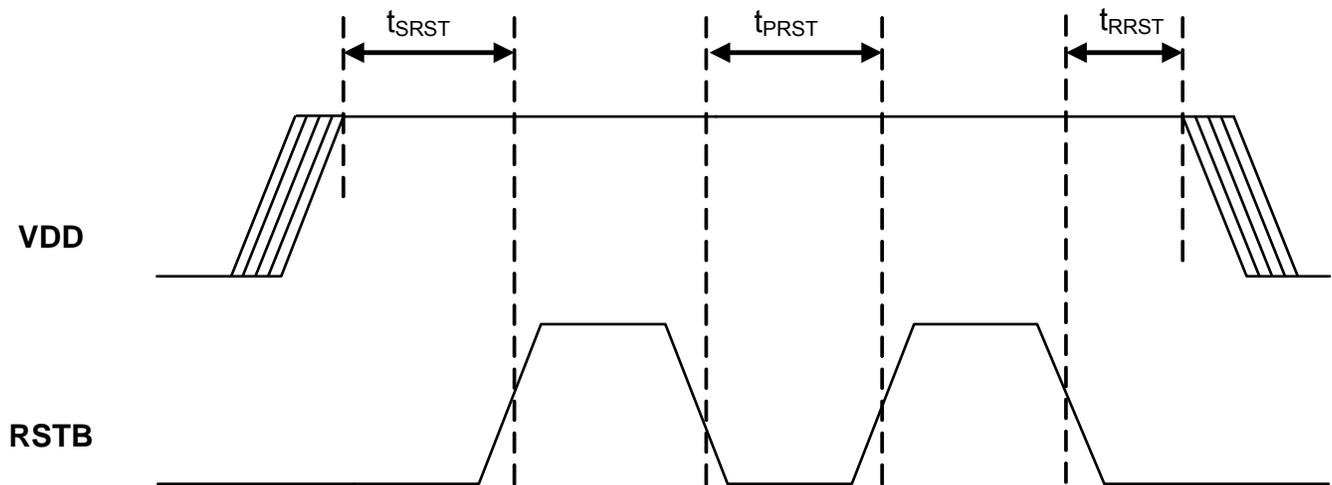
**Figure 1. Reset Timing**
