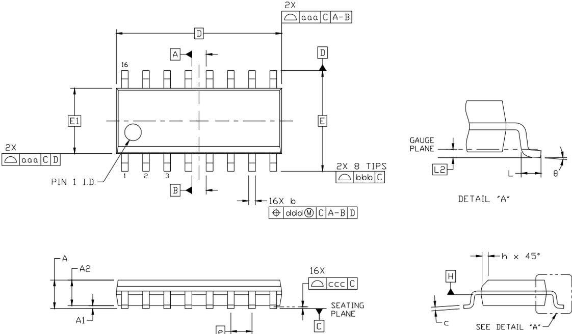
Figure 3. 16-Pin SOIC
