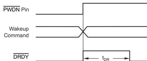
Figure 49. P<sub>WDN</sub> Pin and Wake-Up Command Timing (Pulse-Sync Timing Requirements Shows t<sub>DR</sub>)
