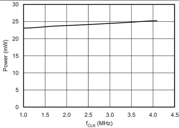
**Figure 20. Power vs Clock Frequency**
