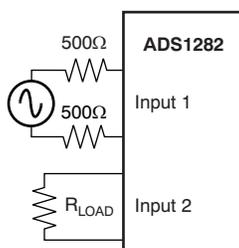
Figure 28. Driving an External Load Through the MUX
