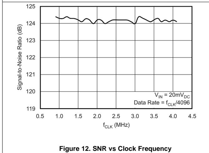
Figure 12. SNR vs Clock Frequency
