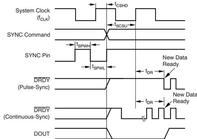
Figure 46. Pulse-Sync Timing, Continuous-Sync Timing With Single Sync
