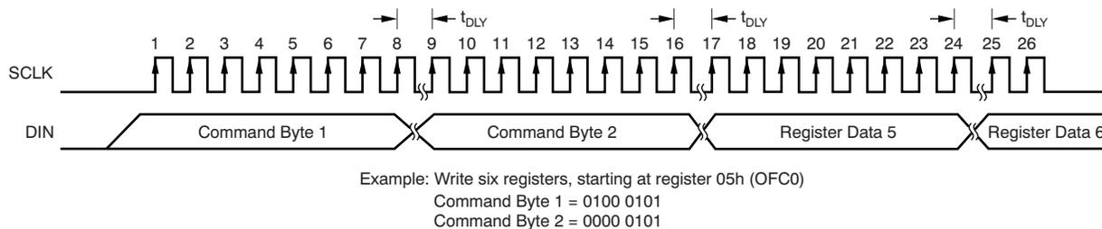
**Figure 60. Write Register Data ( Shows  $t_{DLY}$ )**
