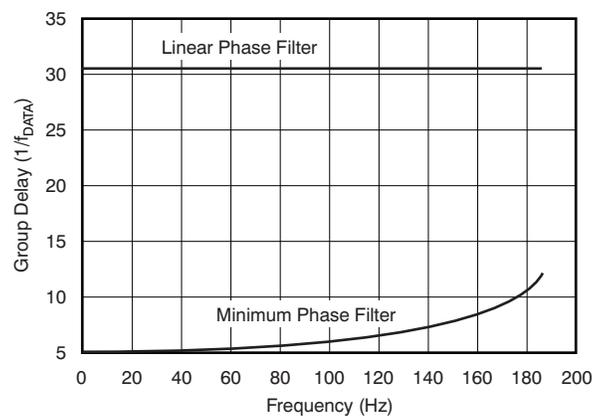
Figure 43. FIR Group Delay ( $F_{DATA} = 500$  Hz)
