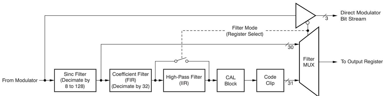
Figure 36. Digital Filter and Output Code Processing
