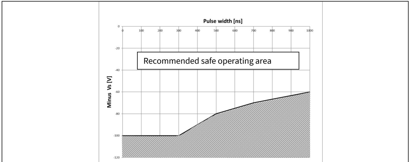
**Figure 18** Negative VS transient SOA for 2ED2101S06F @ VBS=15 V
