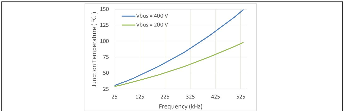
\* Assumptions for above curves: LLC topology, Power switch = IPP60R600P6,  $T_a = 25^\circ\text{C}$ ,  $V_{BUS} = 400\text{ V}$ ,  $V_{CC} = 12\text{ V}$ ,  $R_{gon} = 15\ \Omega$ ,  $R_{goff} = 12\ \Omega$
