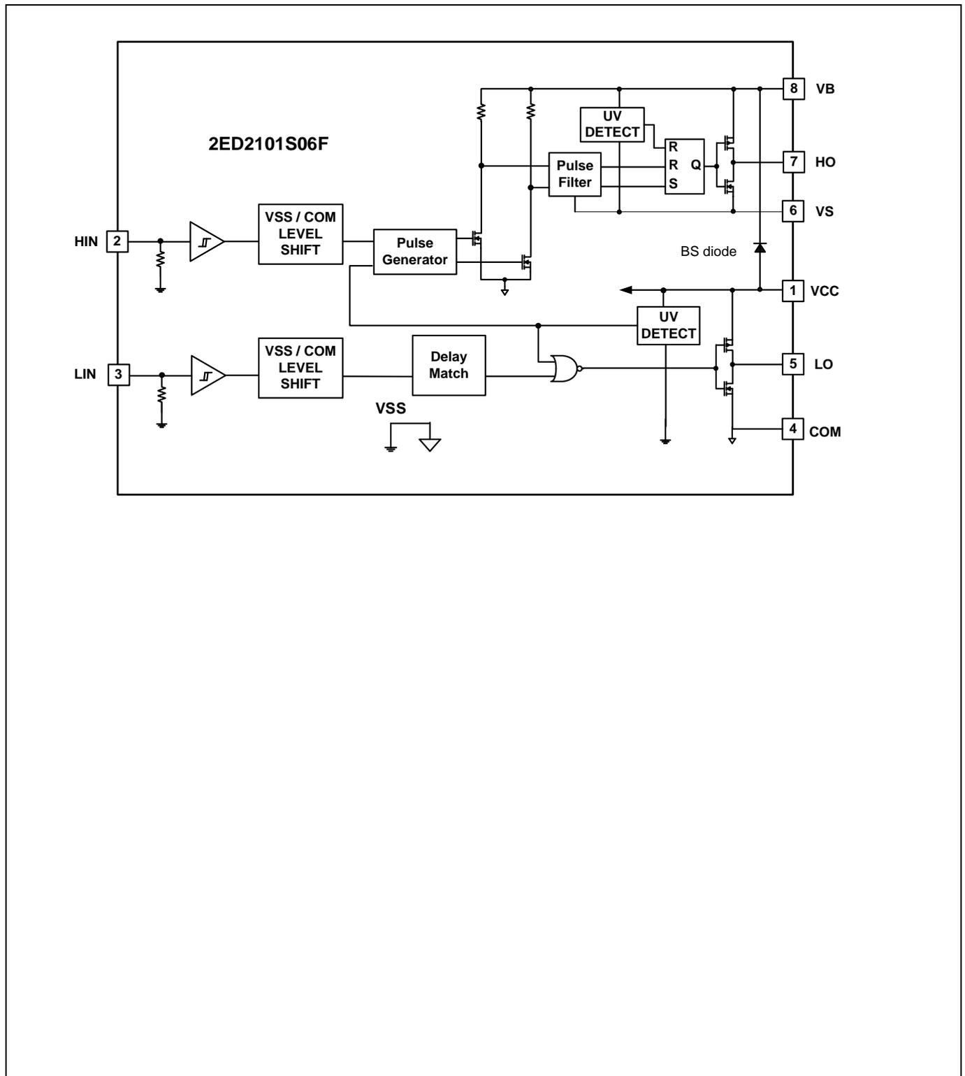
Figure 2 Block diagrams
