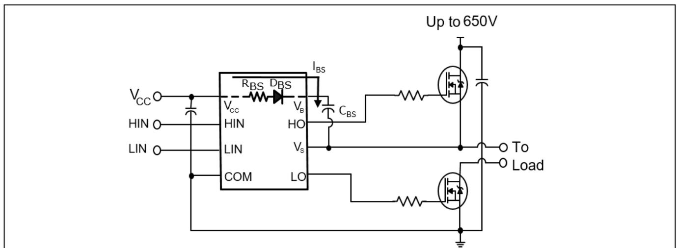
**Figure 13** Half bridge bootstrap circuit in 2ED210x
