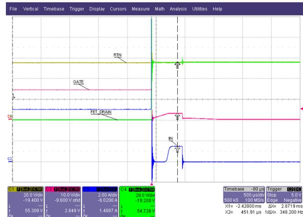
Scope GND = -48V\_B, 5-A Load, After Inductor
