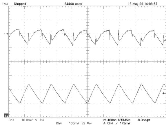
**Figure 11. Positive Output Voltage Ripple in CCM**
