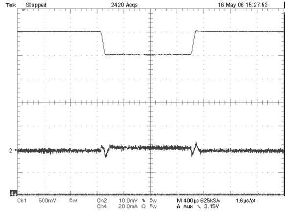
**Figure 6. Line Transient Response  $V_{OUTN} = -5.4$  V, 100 mA**
