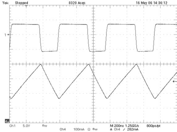
**Figure 9. Continuous Conduction Mode (CCM)**
