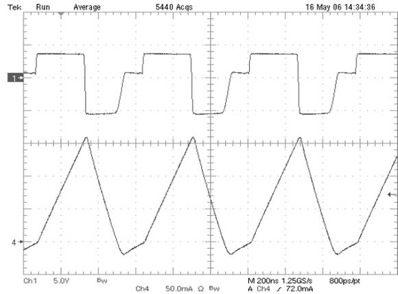
**Figure 10. Discontinuous Current Mode (DCM)**
