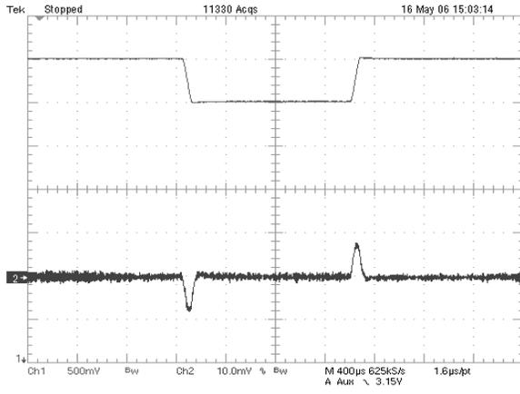
**Figure 5. Line Transient Response  $V_{OUTP}$  at 100 mA**
