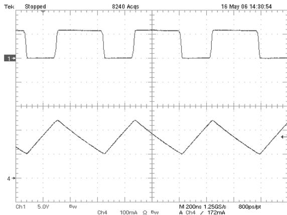
**Figure 7. Continuous Conduction Mode (CCM)**
