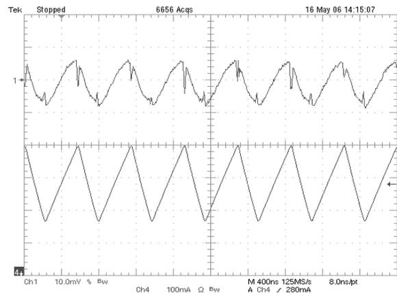
**Figure 12. Negative Output Voltage Ripple in CCM**
