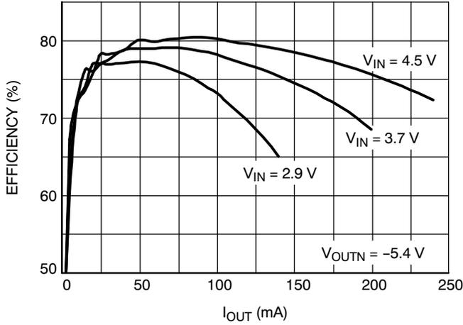
**Figure 3. Efficiency vs.  $I_{OUT}$**
