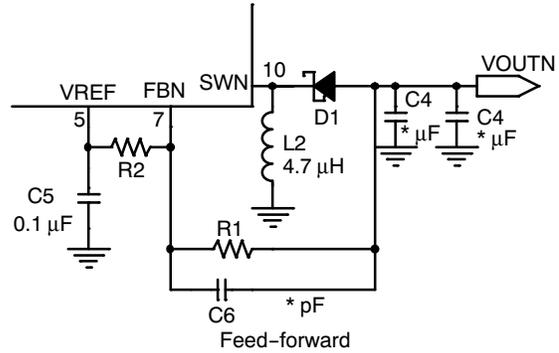
**Figure 15. Inverter Compensation**
