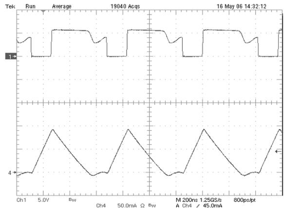
**Figure 8. Discontinuous Current Mode (DCM)**
