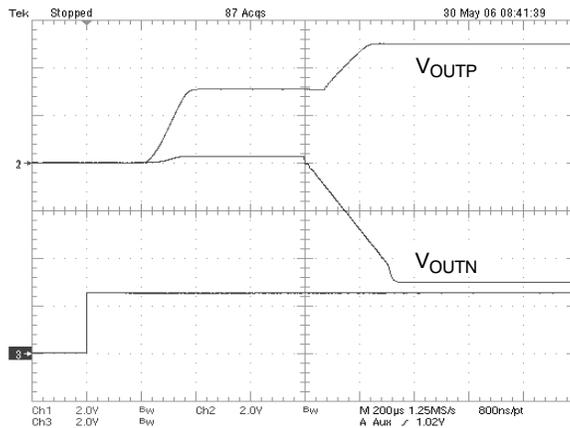
**Figure 13. Start-Up After Enable**
