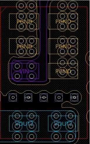
Figure 29. Example of Pad Layout with Vias
