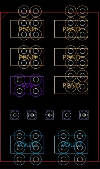
Figure 28. Example of Pad Layout with Vias
