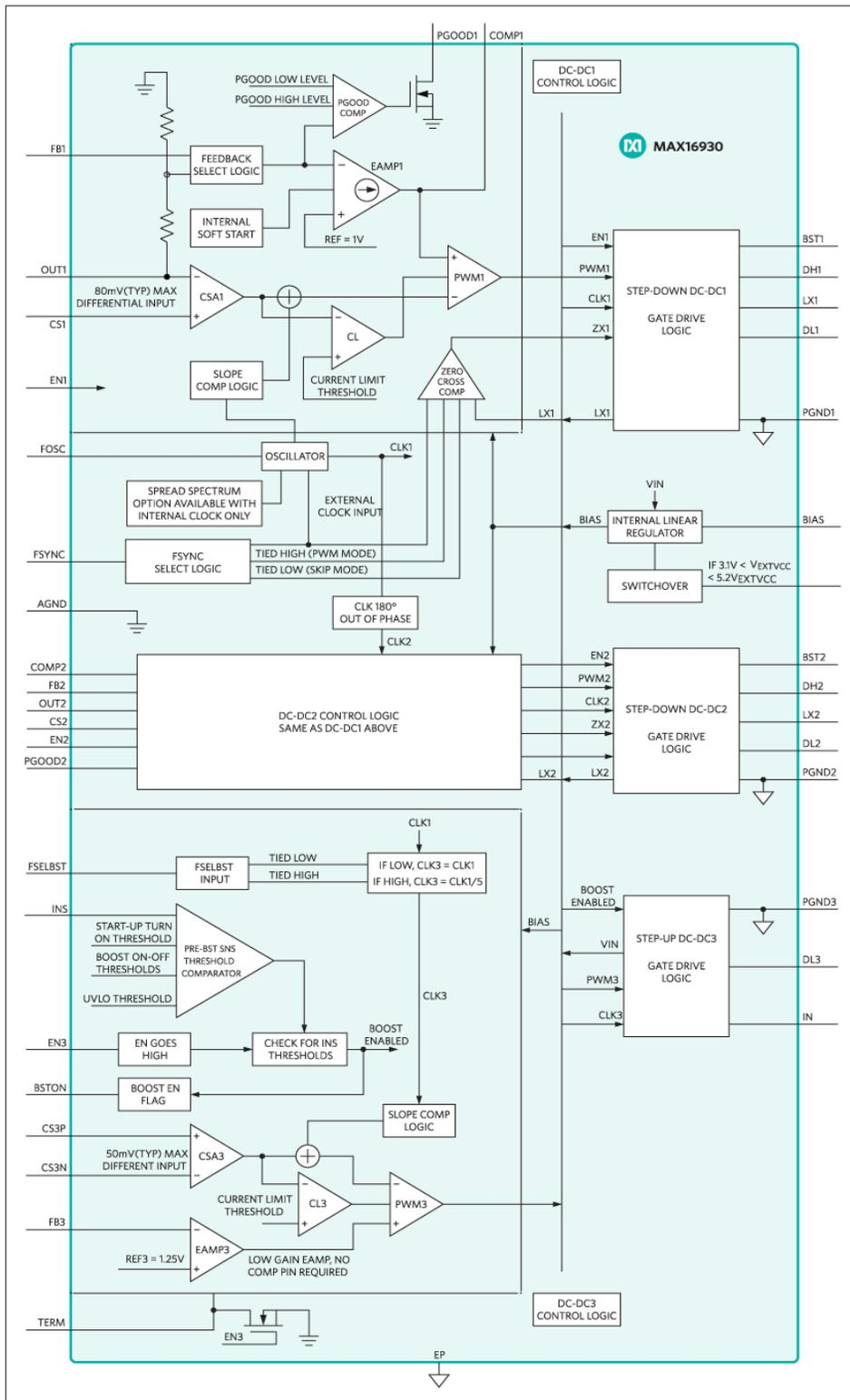
Figure 5. The MAX16930 also provides three outputs, including a preboost for one regulator to ensure that the system operates during cold-crank events, when the rail voltage can drop as low as 2V.
