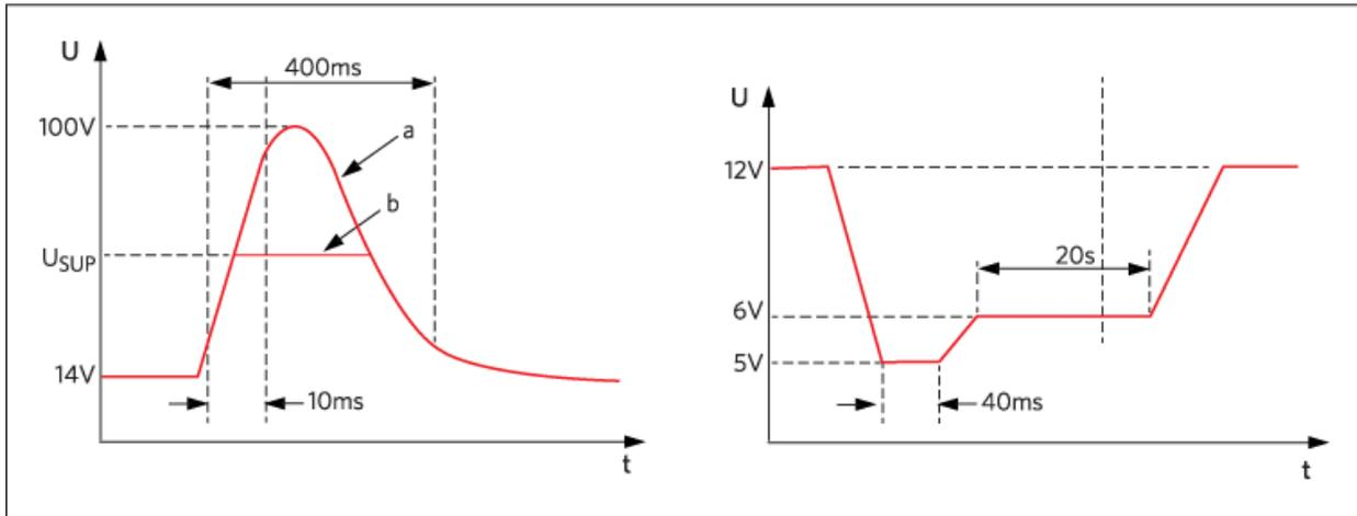
Figure 3. The nominal 12V<sub>DC</sub> battery supply is actually a complex and somewhat hostile electrical rail, as shown by these voltage vs. time characterizations of a) load-dump surge, and b) cold-crank voltage.
