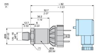
(1) SW24 tightening torque ≤ 25 N.m / 221 lb-in
