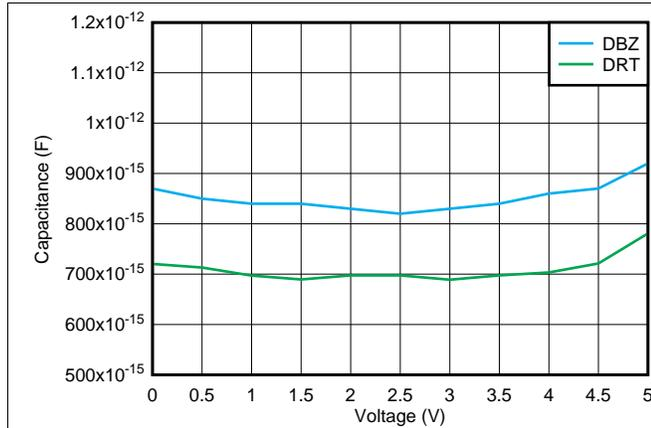
Figure 1. I/O Capacitance vs I/O Voltage ( $T_A = 25^\circ\text{C}$ )
