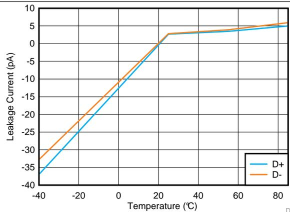
Figure 2. Leakage Current vs Temperature ( $V_{IO} = 2.5\text{ V}$ )
