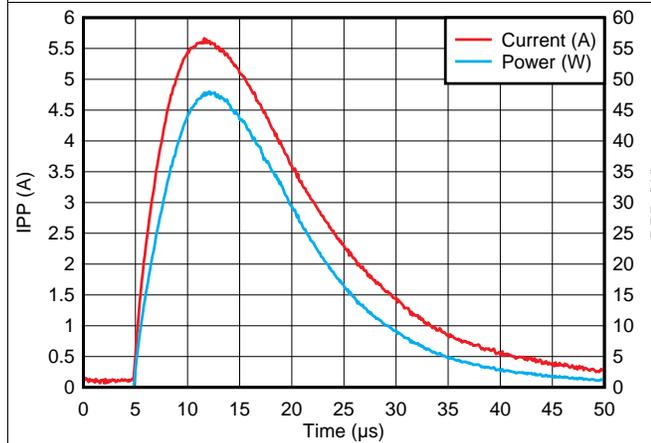
Figure 3. Peak Pulse Waveforms, (Measured at One I/O, With the Other I/O Open)
