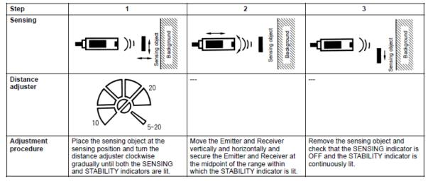
Note: If the STABILITY indicator is not lit while the Sensor is in operation, this indicates a possible operational error. Check or readjust the
