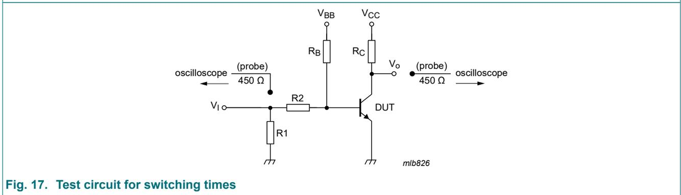
Fig. 17. Test circuit for switching times
