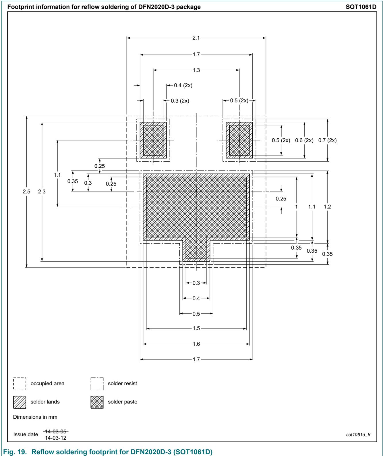
Fig. 19. Reflow soldering footprint for DFN2020D-3 (SOT1061D)
