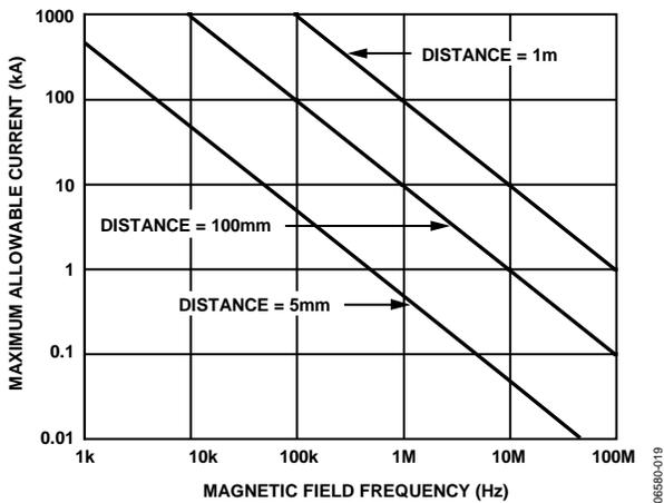
Figure 19. Maximum Allowable Current for Various Current-to-ADuM1410/ADuM1411/ADuM1412 Spacings
