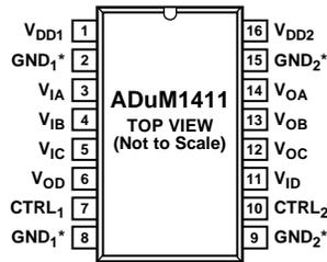
\*PIN 2 AND PIN 8 ARE INTERNALLY CONNECTED. CONNECTING BOTH TO GND<sub>1</sub> IS RECOMMENDED. PIN 9 AND PIN 15 ARE INTERNALLY CONNECTED. CONNECTING BOTH TO GND<sub>2</sub> IS RECOMMENDED.
