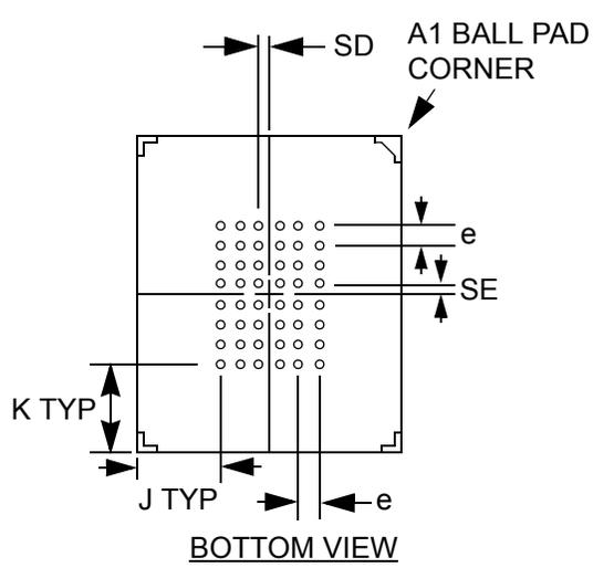
1. DIMENSION IS MEASURED AT THE MAXIMUM SOLDER BALL DIAMETER. PARALLEL TO PRIMARY Z.
